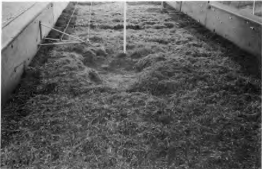
Photo 4 Erosion test 6: Damage after 11 hours of testing
