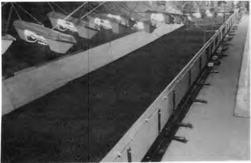
Photo 2 Dike in the Delta Flume prior to testing
