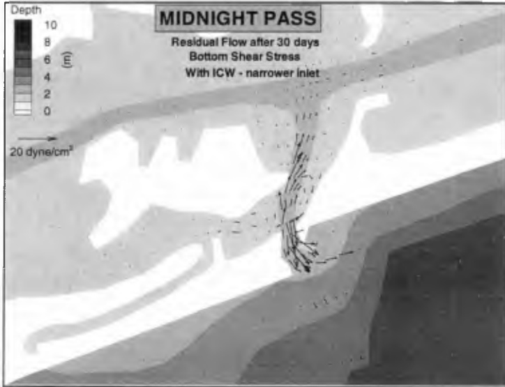
Figure 7 - Residual bottom shear stress over a 30 day simulation with intracoastal waterway and a narrow inlet.
