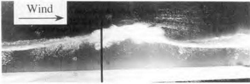
Photo 1. Generation of spray from spilling breaker under strong wind.
