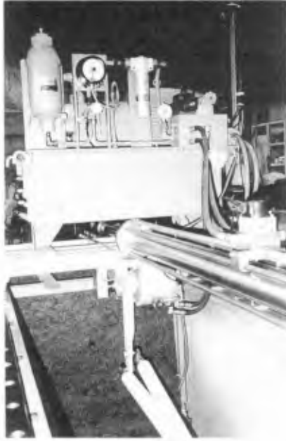
Photo 1. A rotary actuator and cylinder actuator attached to the wavemaker
