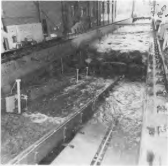
Photo 3 Erosion test 6: H_S = 1.4 m, T_P = 4.7 s
