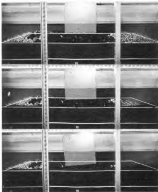
Fig. 7 Settlement of a Caisson Breakwater
