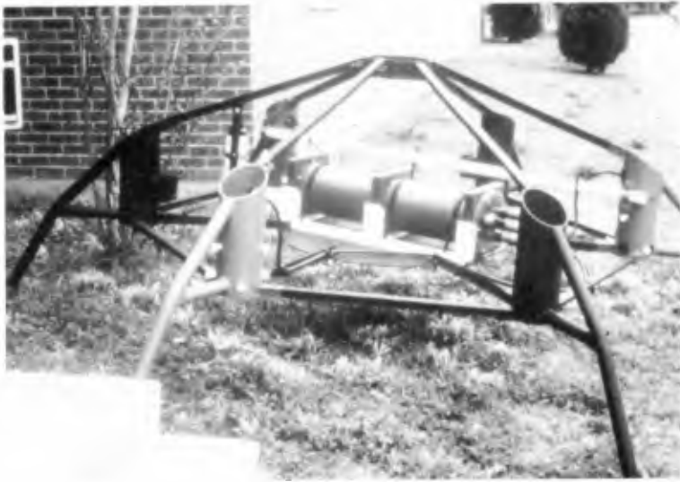
Figure 1: DWG-1 ready for deployment. Base version uses 3 transducers in a 1.6 m equilateral triangle array.
