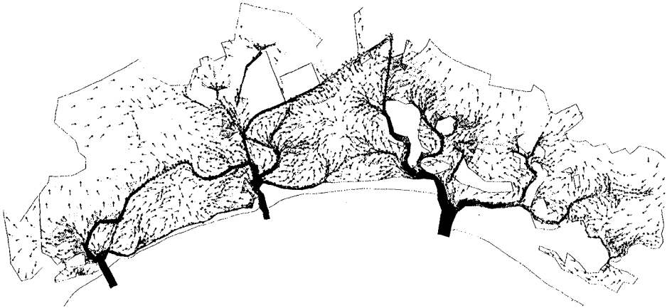
Figure 20. Flow field simulated by the finite element model (4th Feb. 1985 tide; from Cons. Venezia Nuova, REA 1989).
