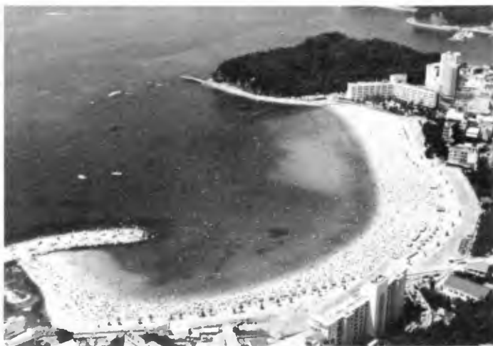
Photo. 1. Present aerial view of stable sandy beach being newly formed in Shirarahama beach after beach nourishment as of 1991
