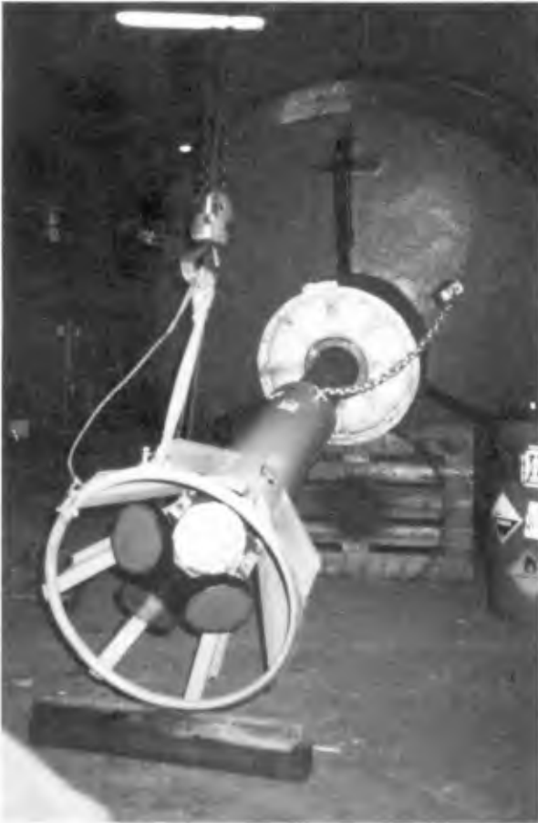
Fig. 7. An ADCP current meter installed below the WAVESCAN buoy.
