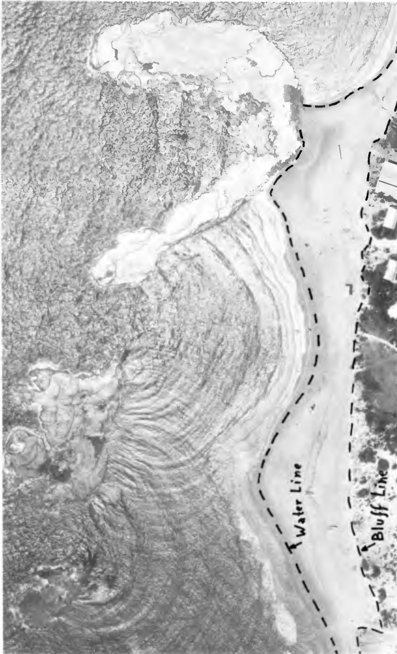
Figure 3 Example of marking of waterline and bluffline on an aerial photograph (Sdot-Yam 31.07.1970)
