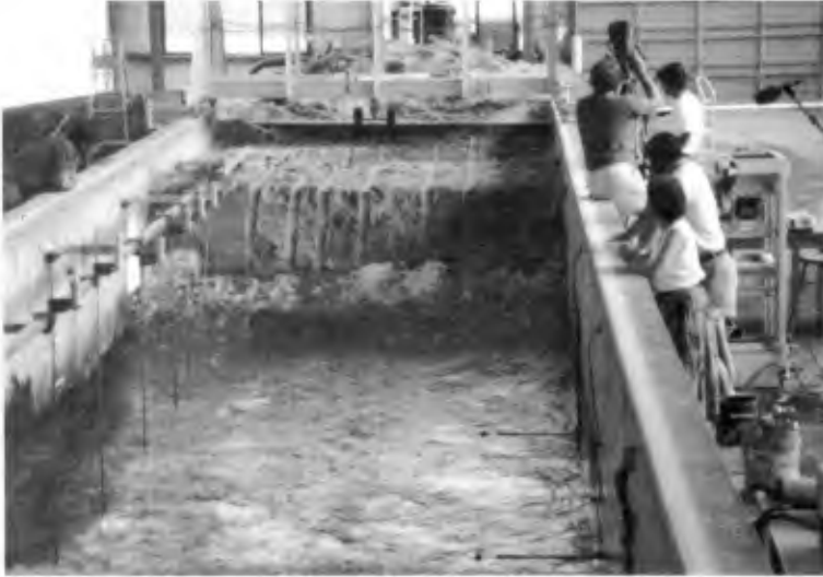
Fig. 3. Capacitance bed surface and water surface gages on the foreshore
