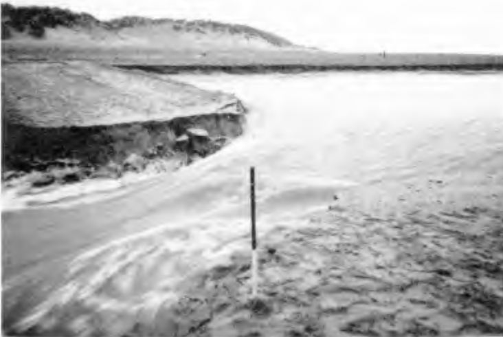
Fig. 7 Photo of breach at t \approx 10 min.
