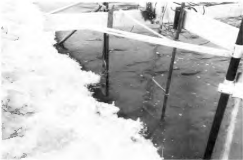
Figure 1. Instrument mounting frame hardware showing typical set-up for measurements in the inner surf zone.
