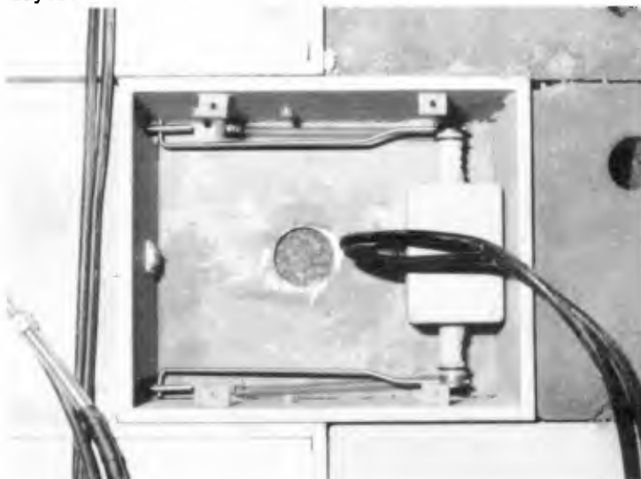
Photograph 2. Displacement gauges in instrumented blocks next to the moving block
