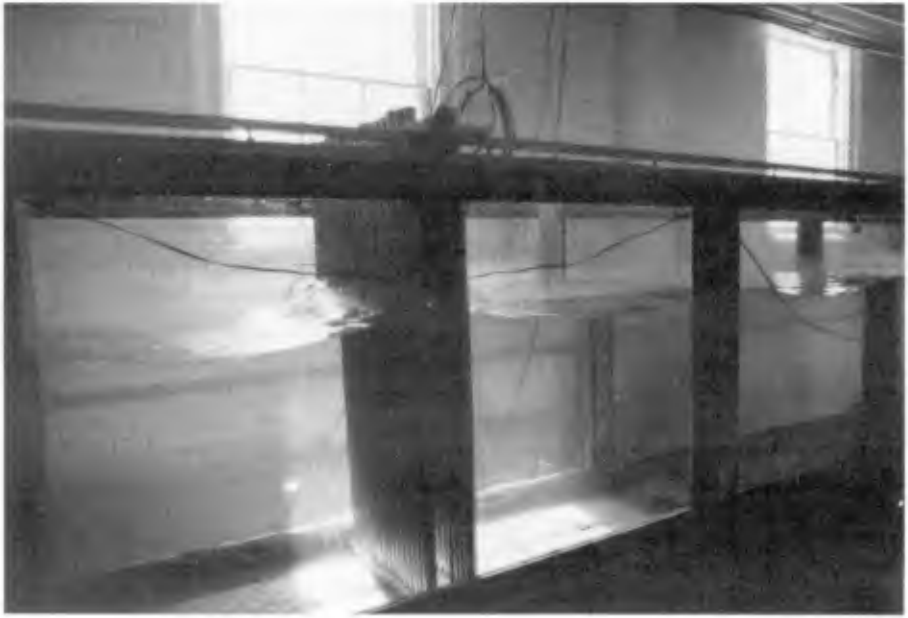
Figure 1. Wave transmission through a pile breakwater in a glass-walled wave channel.
