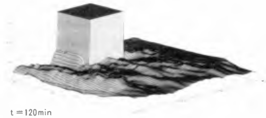
t = 120 \text{ min} Fig.13 Bird's eye view of measured bottom change (Square-I, \theta = 0^\circ , T = 1.0 \text{ s} , H = 10.0 \text{ cm} , t = 120 \text{ min} )
