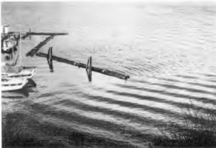
Fig. 3. The log bundle at Reed Point Marina, showing wave reflection and diffraction.
