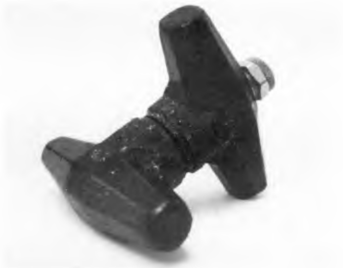
Figure 2 - Current "Load Cell"
