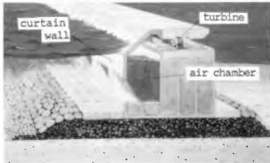
Fig.1 Wave Power Extracting Caisson Breakwater
