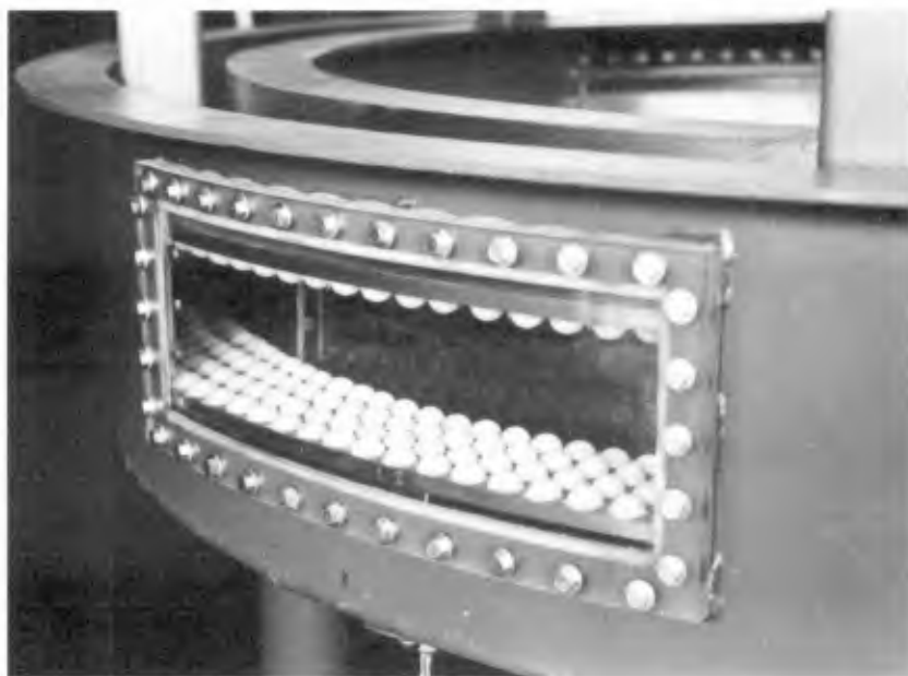
Photo 3 Detail Carrousel: 4 rings of half spheres are glued on the top and bottom ring.
