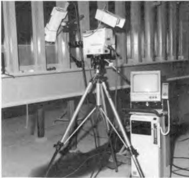
Photo 1 Set-up High Speed Video at Delft Hydraulics Pulsating Water Tunnel.
