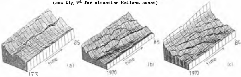
Figure 2. 3-D-time diagram of profile between (a) Den Helder and Petten (b) Petten and IJmuiden (c) IJmuiden and Scheveningen
