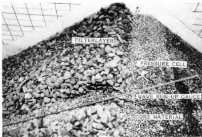
Fig. 6 Pore pressure gauge and wave run-up gauge
