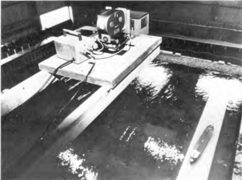
Figure 8. Overhead camera to record model's horizontal excursions
