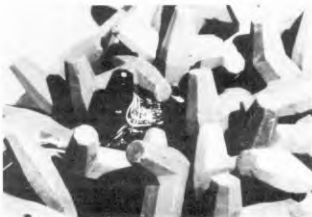
Fig. 11 Example of Instrumented Unit Placement in the Armour Layer
