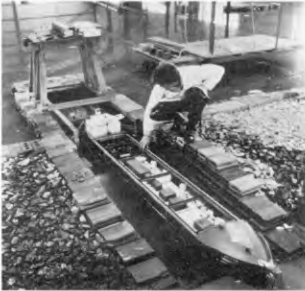
Figure 4. Distribution of lead weights for proper loading
