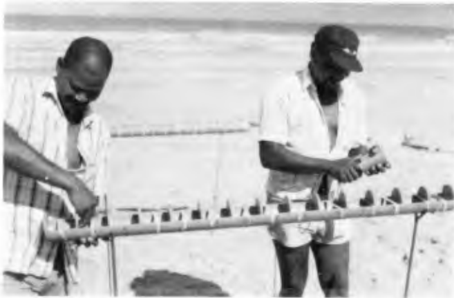
Figure 7. Cleaning of bamboo sampler
