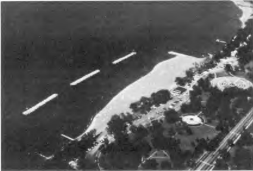
Figure 6. Photograph of Lakeview Park, Lorain, Ohio, shows what can be done with offshore breakwaters and sand fill to form the only good bathing beach for many miles on the Lake Erie shoreline. The cliffs and streams in this vicinity supply very little beach material, and the natural beaches are narrow and not adequate for recreation (Corps of Engineers photograph).
