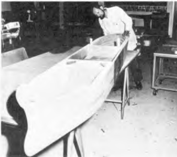
Figure 3. Mould for construction of glass fibre model hull
