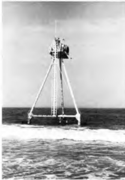
Figure 16 CERC's Coastal Research Amphibious Buggy (CRAB)
