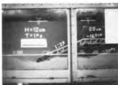
Fig. 14 An example of two dimensional scour
