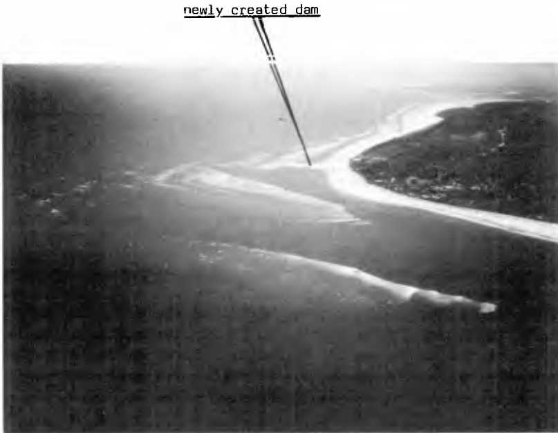
Fig. 4: Aerial view of the newly created connection of the offshore bar to the beach of the Isle of Langeoog by means of a sand dam.
