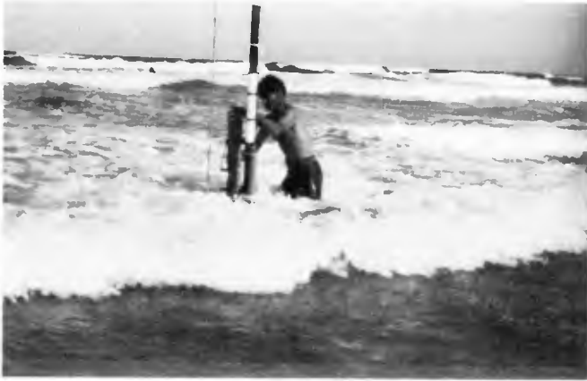
Figure 6. Replacing bamboo sampler at measuring stand
