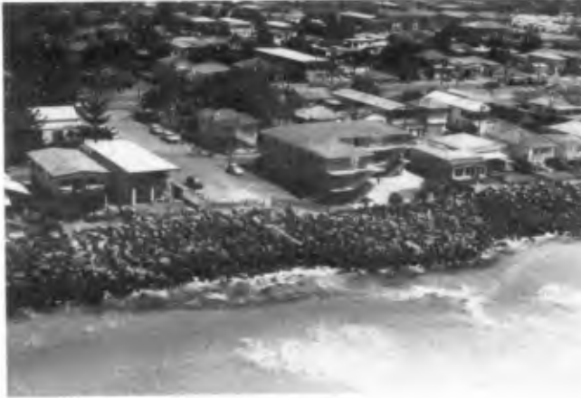
Palm Beach in 1980 with residential development protected by rock seawall and no usable beach.
