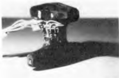
Fig. 6 Instrumented Dolos Unit
