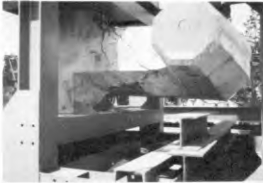
Photograph 4: The cracks of the stem (Static load test)
