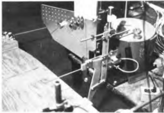
FIG.8 PHOTOGRAPH SHOWING THE CANTILEVER SPRING, FENDER, AND MOORING FORCE TRANSDUCER
