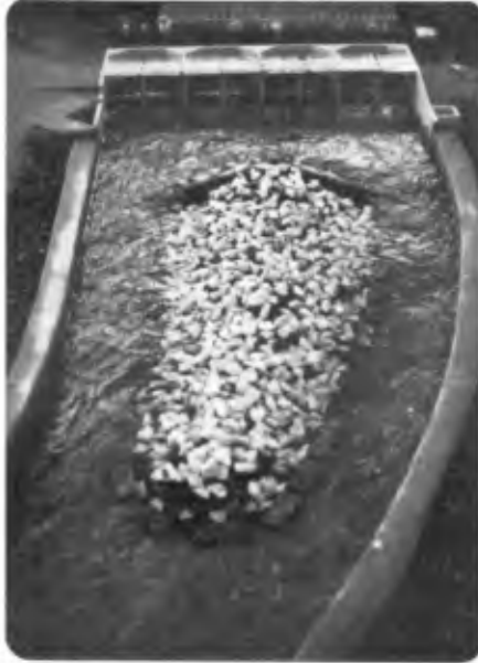
5: MODELLED WAVE ENERGY DISSIPATOR (SWL -0,5 m GMSL, flow 80 cumecs)
