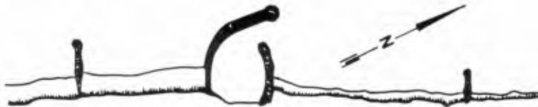
Fig. 8. A map of Ziqim Harbour, drawn from an aerial photograph. Note the extreme widening of the beaches to the north. These are now almost totally exposed of their sand cover gearround. Prior to harbour construction beaches to the north had normal sand quantities and normal widths even during severe winter storms.
