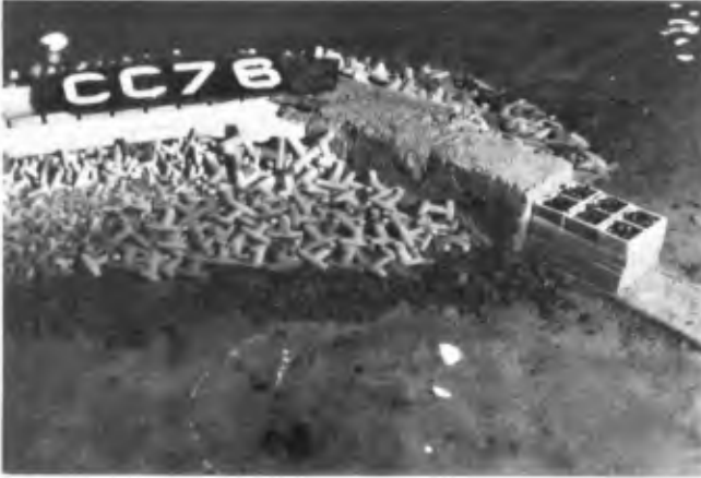
Fig. 7 Typical 7 layers placed in 3 columns unstrapped filled with gravel (simulating concrete)
