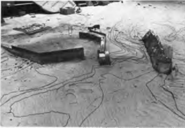
Fig. 6 Build-up in model sand trap
