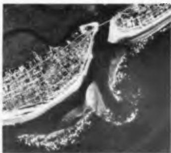
Figure 8. Vertical aerial photograph of Breaches Inlet, South Carolina showing that a new channel has recently been breached through the ebb-tidal delta. The abandoned channel is being filled with sediment at this time.
