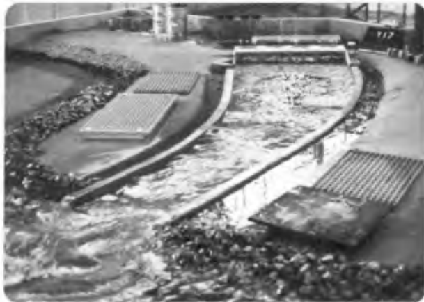
6: MODELLED WAVE ENERGY DISSIPATOR (SWL +1,0 m GMSL, flow 80 cumecs)
