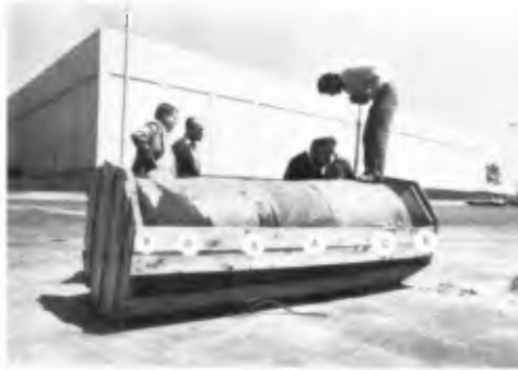
PROTOTYPE TESTING OF SAND COATED TUBES USING A HUNTING KNIFE
