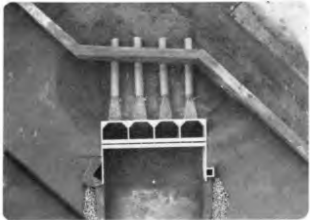
2: CLOSE-UP VIEW OF MODEL OUTFALL STRUCTURE
