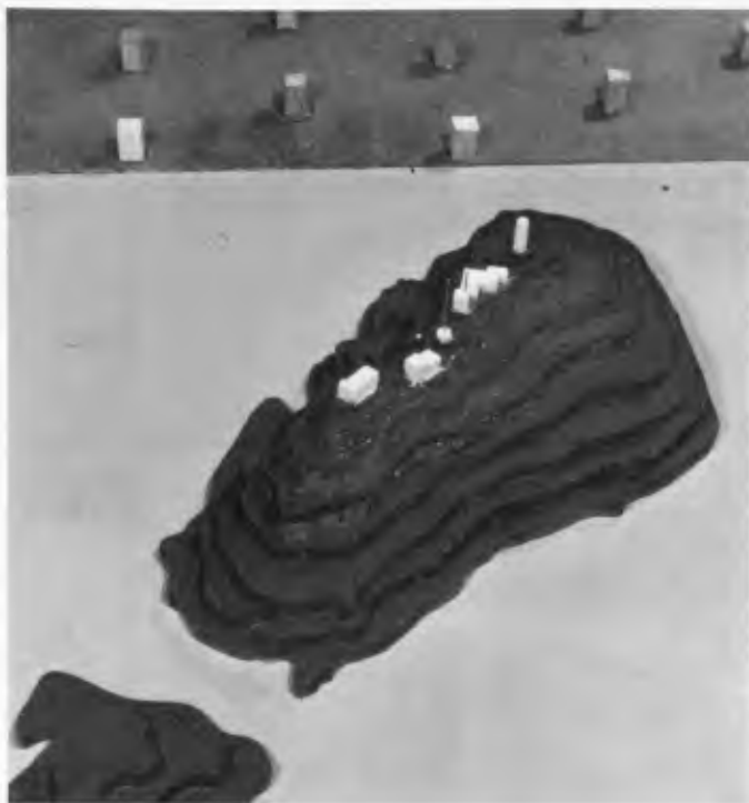
FIG. 1 1/600 scale wind tunnel model of Waglan Island used to determine anemometer position error corrections.
