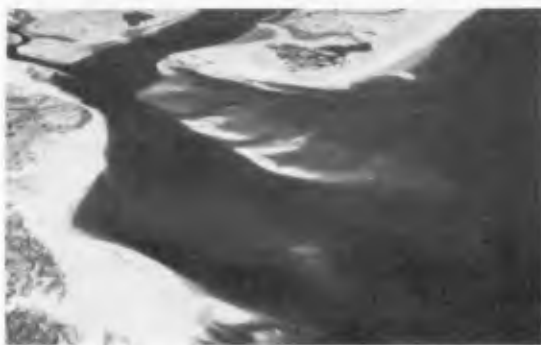
Figure 10. Oblique aerial photograph of Parker River Inlet, Massachusetts. Note that the main ebb channel abuts the downdrift beach and that the bulge in the downdrift shoreline coincides with bar welding.
