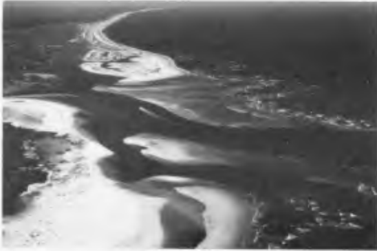
Figure 23. Oblique aerial photograph of Murrels Inlet, South Carolina. Inlet sediment bypassing at this inlet occurred through ebb-tidal delta breaching prior to being jettied.
