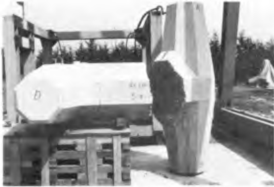
Photograph 5: The breakage of Dolos (Drop test)
