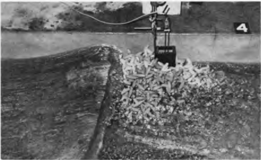
FIG. 7 FLUME TEST ON 'HALF MODEL' 7 M BREAKING WAVES
