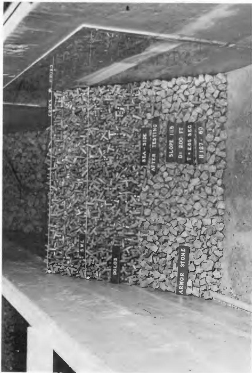
Photograph 3. Pattern 1 after attack of 2.65-sec, 18.5-cm waves
