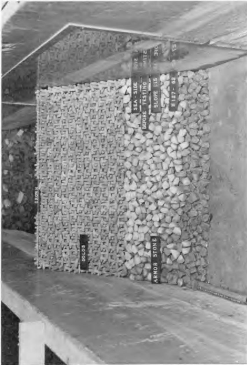
Photograph 8. Pattern 3 with two layers of armor units in place
