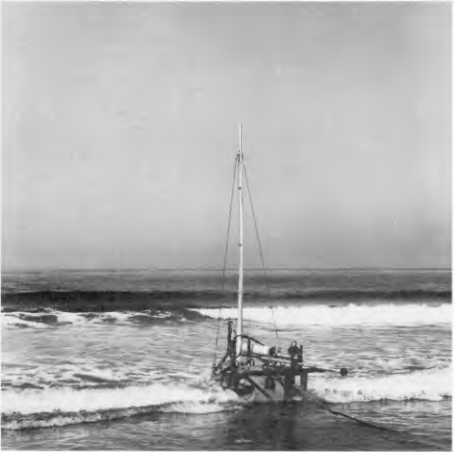
THE PROFILER ENTERING THE SURF ZONE ON A CALIBRATION TRIAL. THE STADIA ROD IS MOUNTED FOR CALIBRATION PURPOSES ONLY AND IS NOT NORMALLY USED WITH THE PROFILER.
