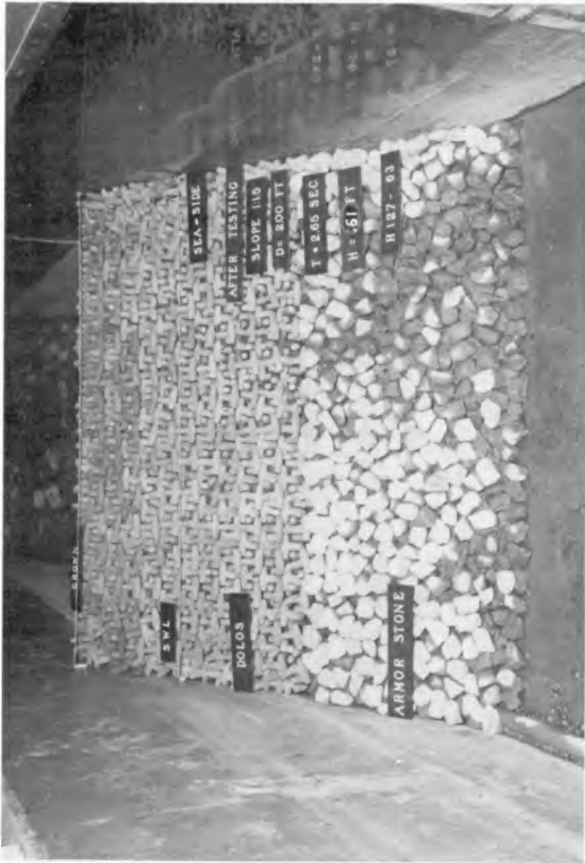
Photograph 9. Pattern 3 after attack of 2.65-sec, 18.5-cm waves
