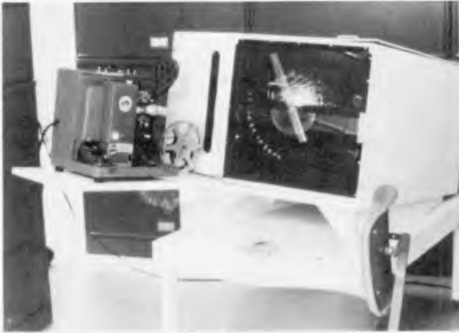
Figure 11. Device used for the analysis of radar film.
