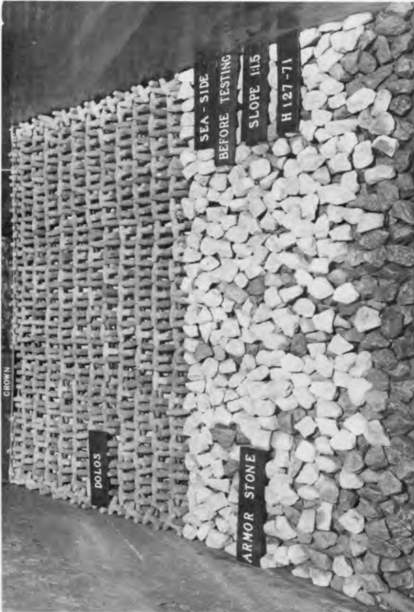
Photograph 5. Pattern 2 with two layers of armor units in place
