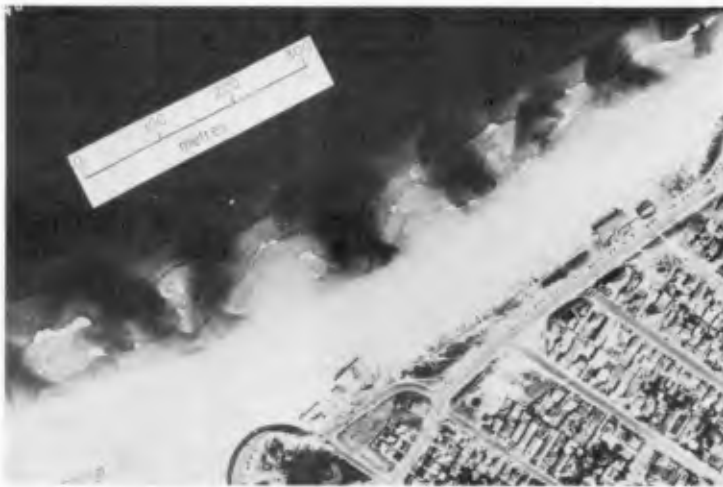
Figure 12 : Rhythmic transverse bars and rip embayments of Type 4 topography (Cronulla Beach, N.S.W.)
