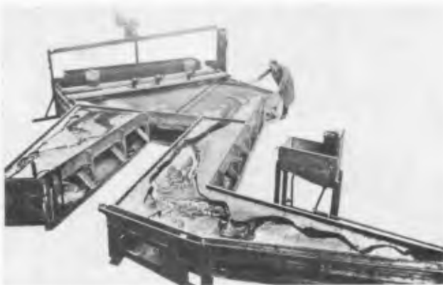
Fig.3 MERSEY, DEE AND LIVERPOOL BAY MODEL Horizontal Scale 1:7040 Vertical Scale 1:190
