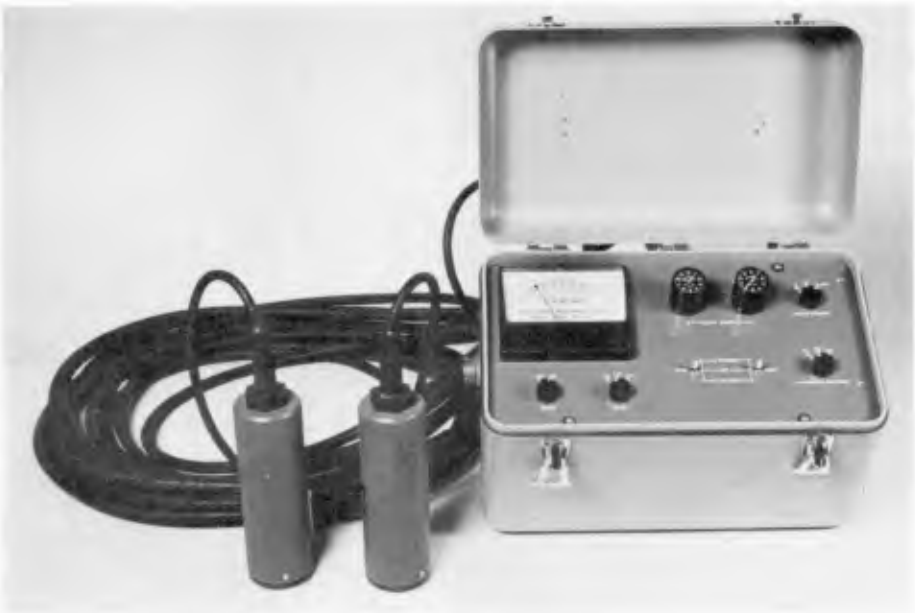
Figure 4. Wave/fluid mud pressure-sensing device (recorder not shown).
