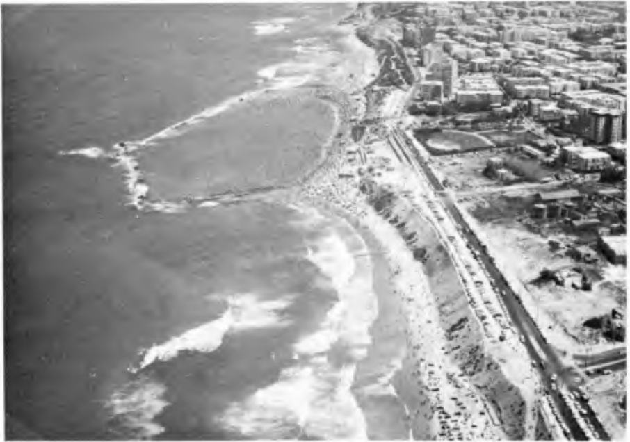
Fig. 5. Sela Beach. Difference in Agitation Between Inside and Outside the Enclosed Area. Limited Bathing Outside.
