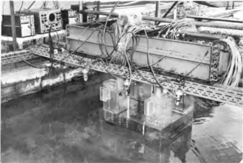
FIG. 7 Model Berth Caisson and instrumentation
