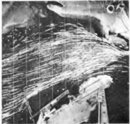
Photo 6. Harbour Protection with Deflector
