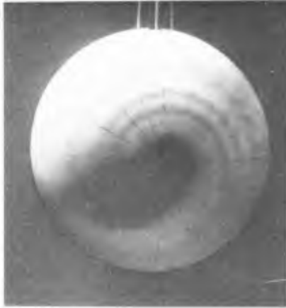
Figure 5. Dye spreading in a spiral from the side port towards the vertical equator at \pi d_0/D = 1.1 . Waves progressing from left to right.
