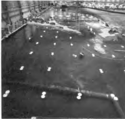
Photo 2. Churchill Tidal Model with Supply Manifold in Foreground, and a Dam Past the Dock.
