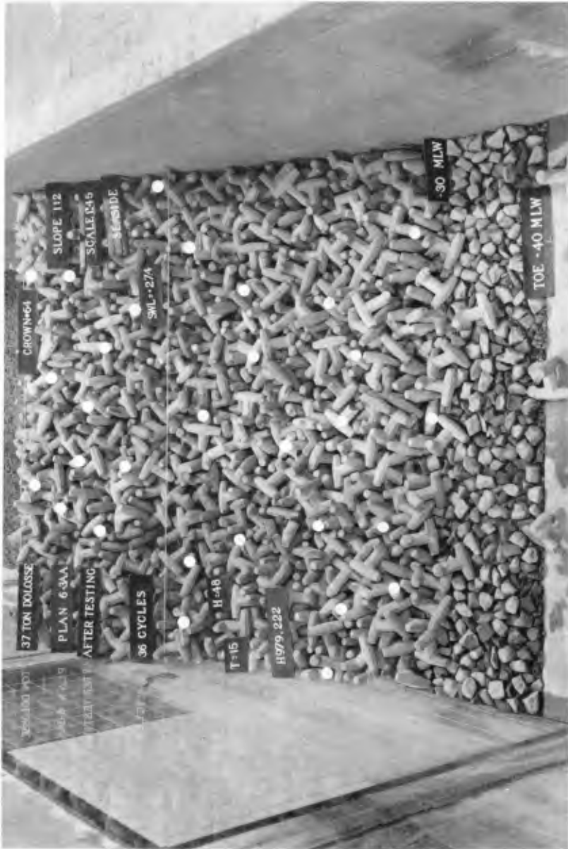
Photograph 7. Test section with 10 percent of the top layer of dolosse broken and uniformly distributed after testing with an extreme wave condition of 15-sec, 48-ft waves at a swl of +27.4 ft msl.
