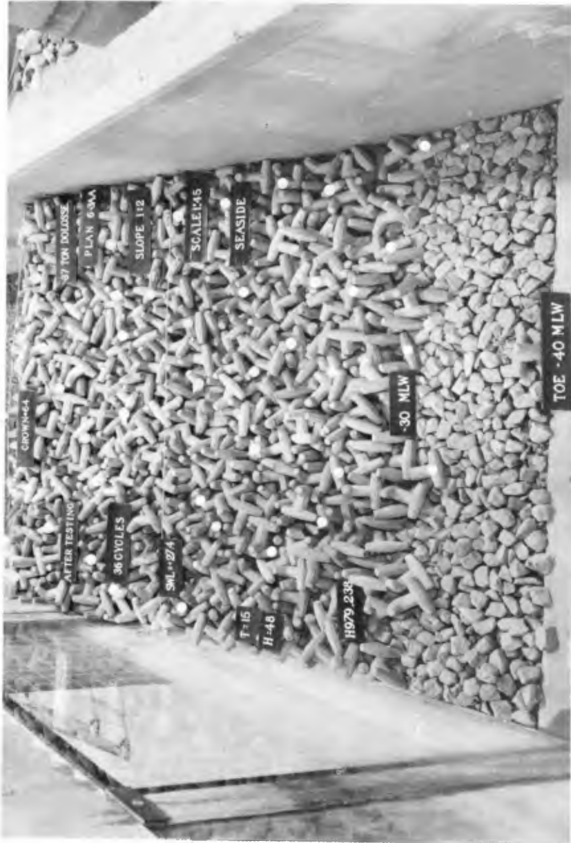
Photograph 8. Test section with 15 percent of the top layer of dolosse broken and uniformly distributed after testing with an extreme wave condition of 15-sec, 48-ft waves at a swl
