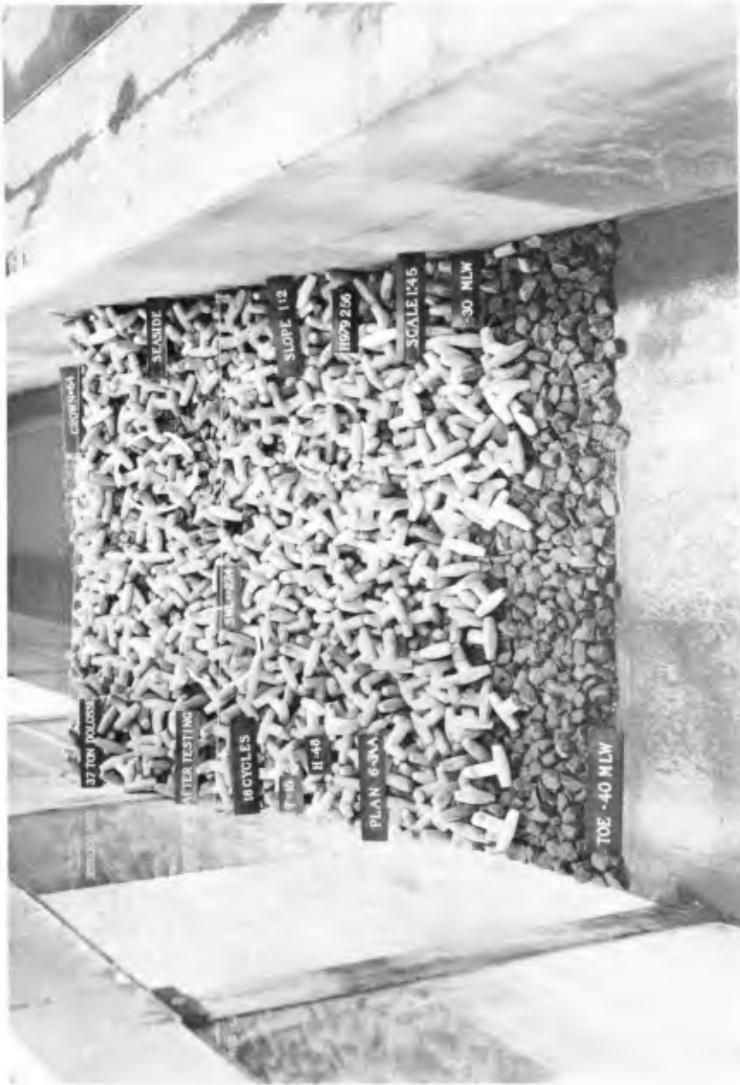
Photograph 10. Test section with 10-unit clusters broken after testing with an extreme wave condition of 15-sec, 48-ft waves at a swl of +27.4 ft mlw.
