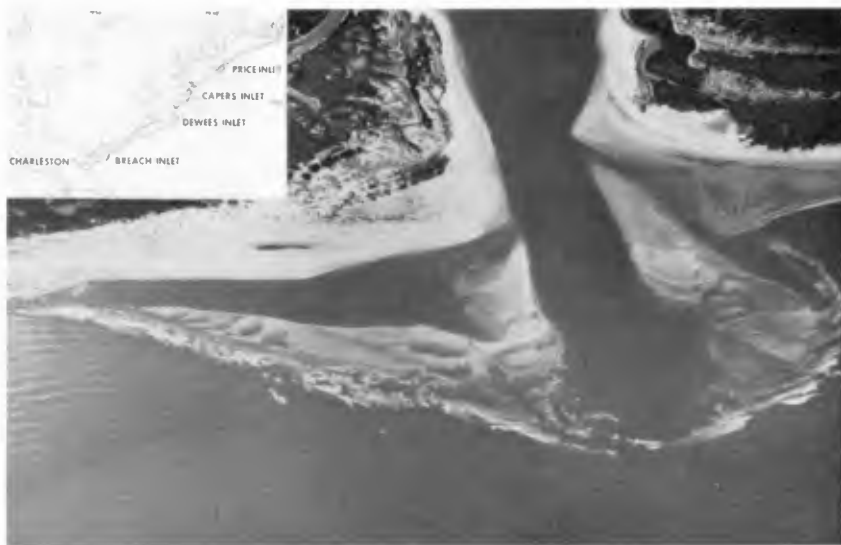
Figure 1. Aerial view and location map of Price Inlet, South Carolina. Note the well-developed ebb-tidal delta.
