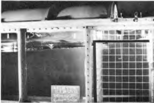
Fig. 6. Standing wave outside and inside the wave chamber of a perforated vertical wall breakwater
