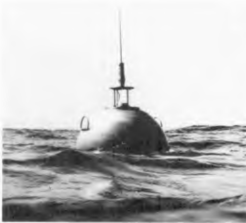
Fig.3 - DATAWELL type accelerometer buoy (Sines, 19th Sept. 1971).
