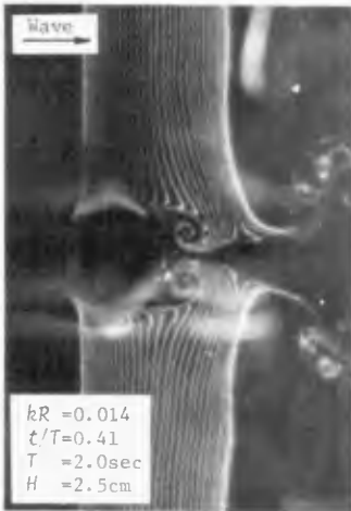
Photo.4 Occurrence of wake vortices behind pile due to waves. (R=1cm)
