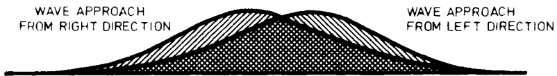
Fig. 4: Changing of the form of the spit due according to the prevailing wave direction
