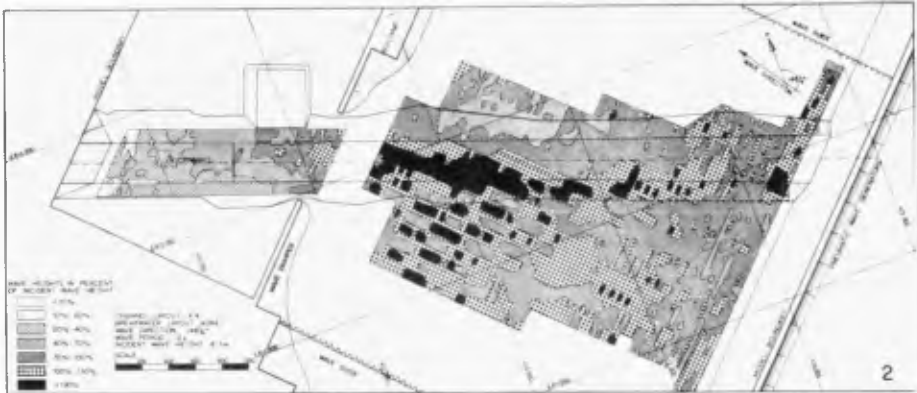
Fig. 7. Relative wave heights in entrance channel without breakwaters.
