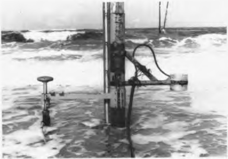
Figure 3: Installation of a two-component electromagnetic current meter and a pressure cell protected against seawater
