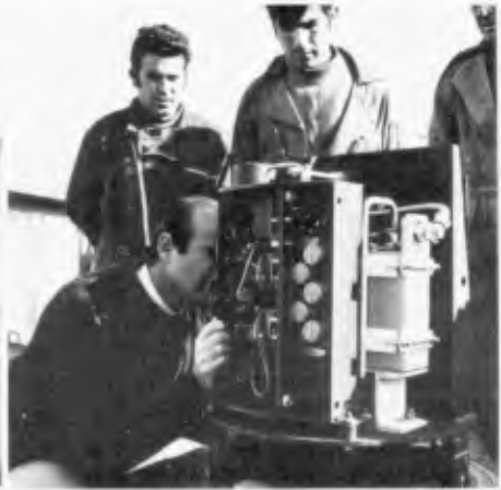
Fig.9 - Adjustment of pressure wave recorder (Huelva).
