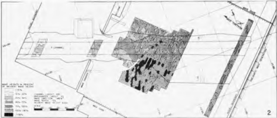
Fig. 11. Wave penetration diagram, 1:100 slope, 146\frac{0}{4} , 12 s waves
