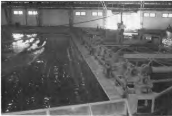
Fig. 3.1. The Plunger-Type Wave Generator
