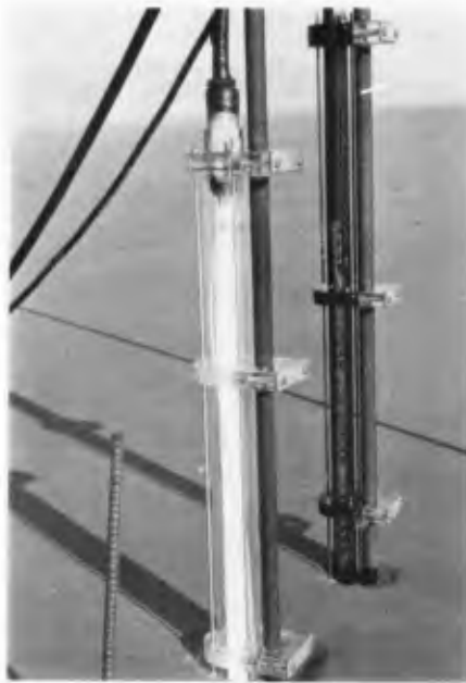
Figure 1. The almometer emplaced on the beach. The device consists of two acrylic cylinders; in one is a fluorescent lamp in the other, 64 photo-electric cells.
