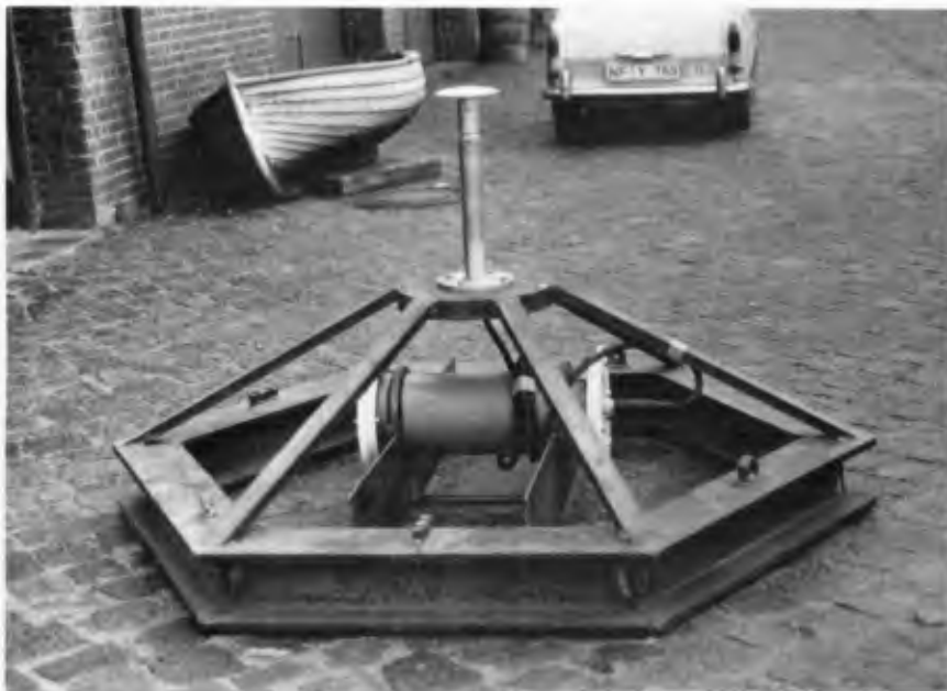
Fig. 3. COMEX electromagnetic current-meter, mounted on its support
