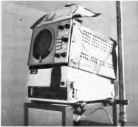
Fig.13 - Huelva radar (block and sighter).
