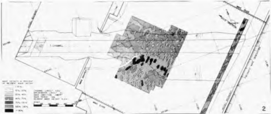
Fig. 15. Wave penetration diagram, short kink breakwater, 146\frac{1}{2}^{\circ} , 12 s waves.
