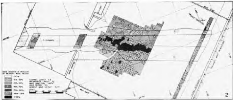
Fig. 10. Wave penetration diagram, 1:60 slope, 146\frac{0}{4} , 12 s waves.
