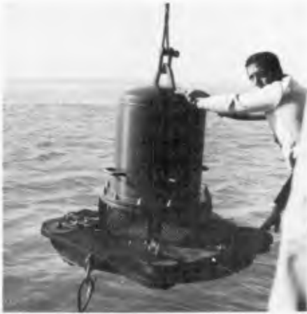
Fig.8 - CHATOU type pressure wave recorder (experimental stage in January 1965 at the Tagus estuary).
