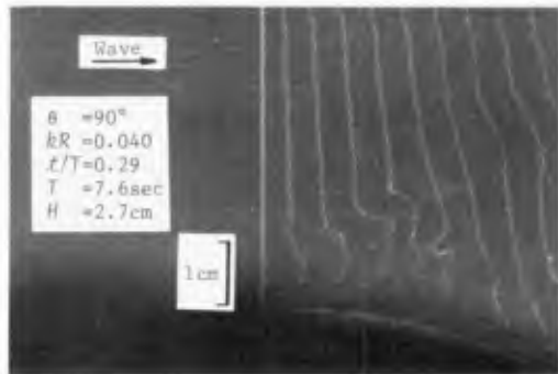
Photo.1 Hydrogen bubble lines in boundary layer.
