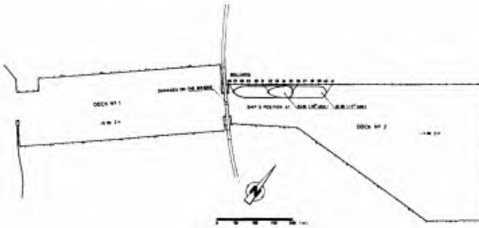
Fig. 16 - Damages on the bridge
