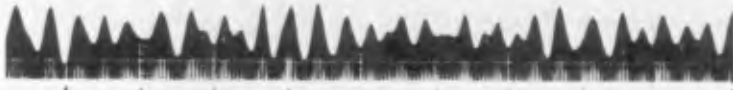
Fig.10 - Typical record of pressure wave recorder (Lagoa de Albufeira, 5th October 1965 at 22.09h. T_C = 10.28s ; H_S = 1.79m ).
