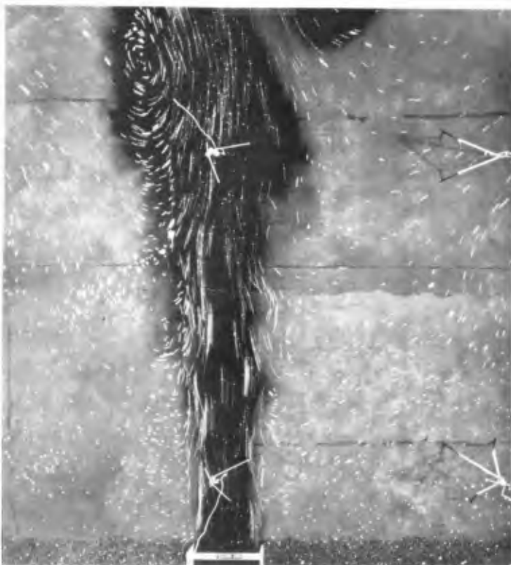
FIG. 7-EBB CURRENT EMANATING FROM THE INLET AND DIFFUSING AS A TURBULENT FREE JET IN THE OCEAN
