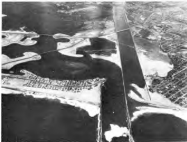
NAVIGATION AND FLOOD CONTROL CHANNELS MIDDLE JETTY CLOSED, CREATING TWO CHANNELS SEPT. 1951
