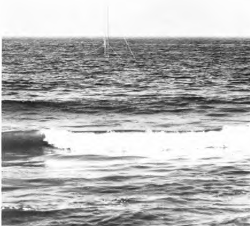
Fig. 2. One of the three identical cup anemometer arrays located on a fixed offshore mast in the area between the outer and the inner bars on the coast of the Gulf of Mexico near Fort Walton Beach, Florida. Two resistance-wire wave gages are shown in the background.
