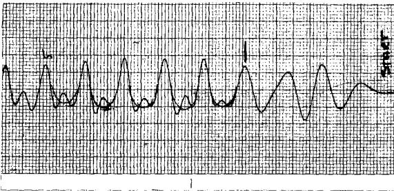
FIGURE 7. Recorded data (9' from wavemaker) Note presence of first harmonic. Test Condition: h = .833' , T = 1.18 sec., |n|/(S/2) = .109 (not to same scale as above) a = .52' , (S/2) = 1'' .
