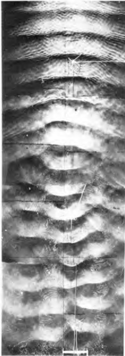
FIG. 12-WAVE TRAIN PROPAGATING ONTO AN EBB CURRENT. U/c_0 = 0.101 , L_0/d = 4.58 , H_0/L_0 = 0.028
