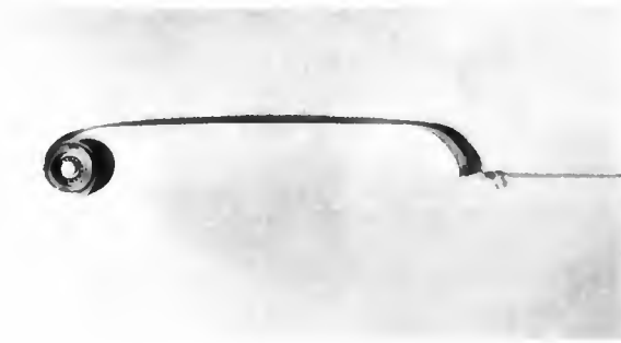
Fig. 8. Special Coil Spring with Constant Reaction
