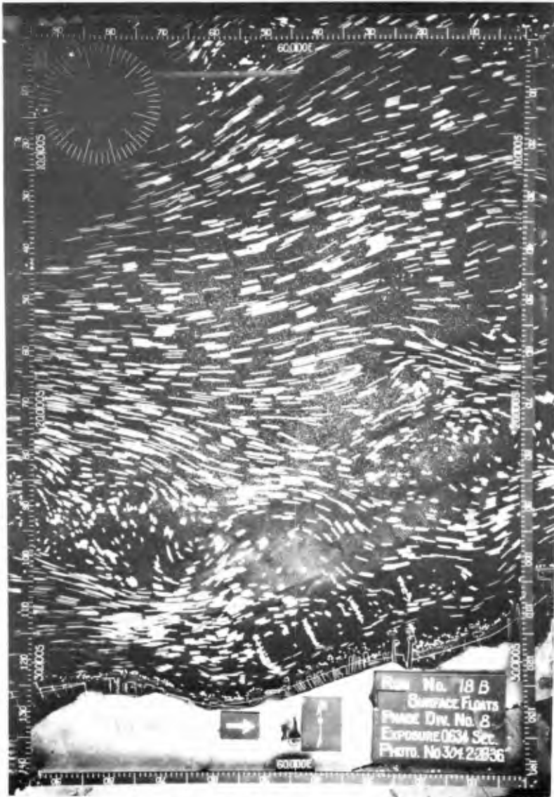
Fig. 5. Typical photograph for measurement of surface currents in the model.
