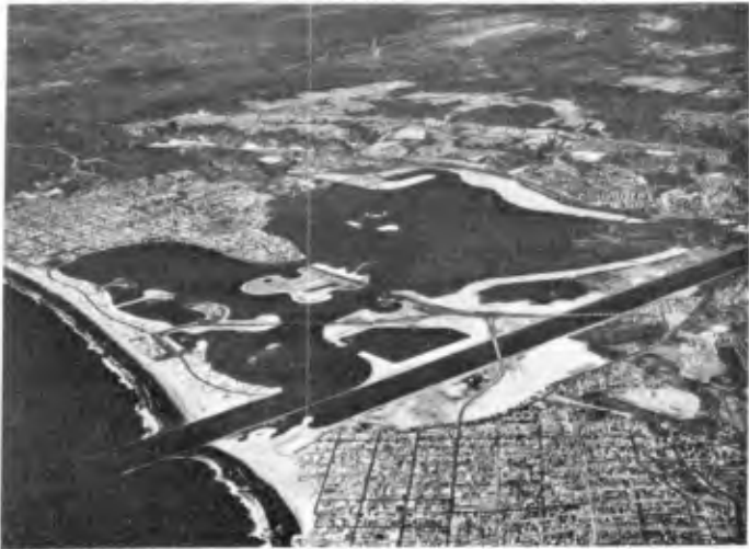
START OF DEVELOPMENT OF EAST MISSION BAY NOTE COMPLETED DREDGING OF ENTRANCE CHANNEL JAN. 1958 NO. 8
