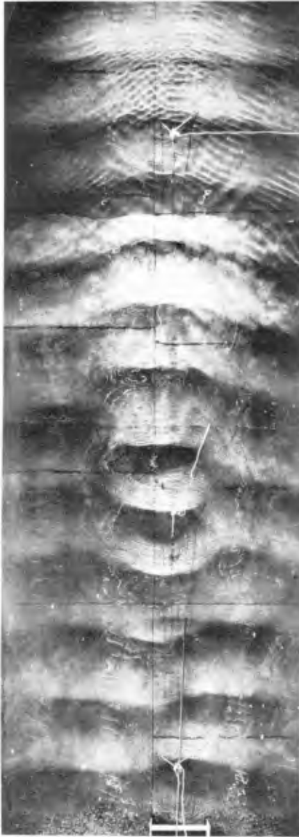
FIG. 11-WAVE TRAIN PROPAGATING ONTO AN EBB CURRENT. u/c_0 = 0.097 , L_0/a = 5.37 , H_0/L_0 = 0.021
