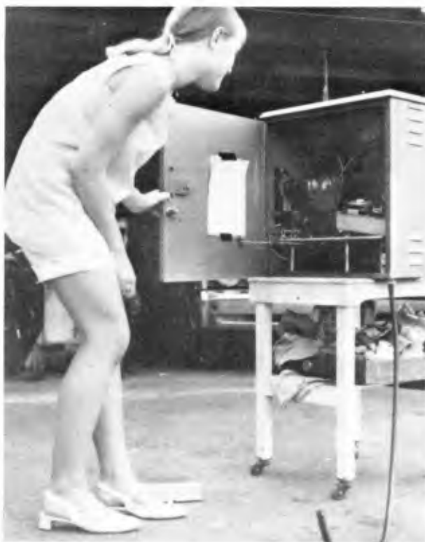
Fig. 11. Photograph of assembled U. S. Army Engineer District, Los Angeles, time-interval camera and accessories in enclosure
