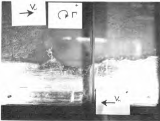
Breaking of the Crest Produced by too Much Applied Circulation
