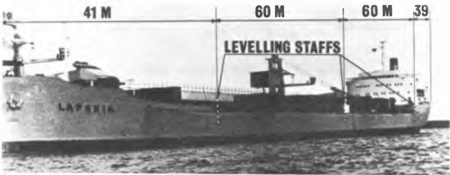
FIG. 4 LEVELLING STAFFS ATTACHED TO SHIP
