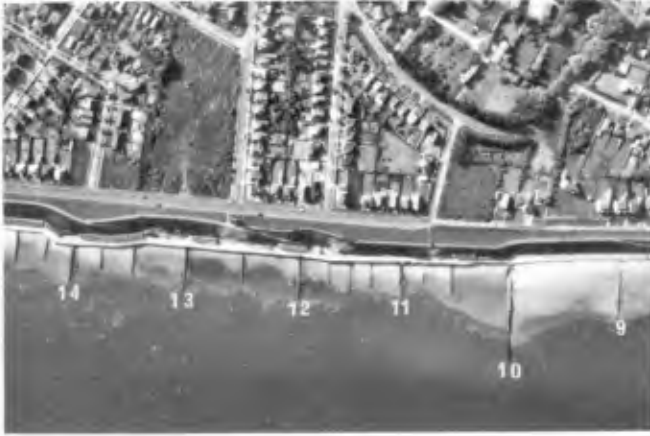
Fig. 4: Part of the frontage with large groyne No. 10 (Distance between numbered groynes 100 m.)
