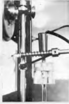
Fig. 12 - Servo-coordinograph. Detail of the recorder.
