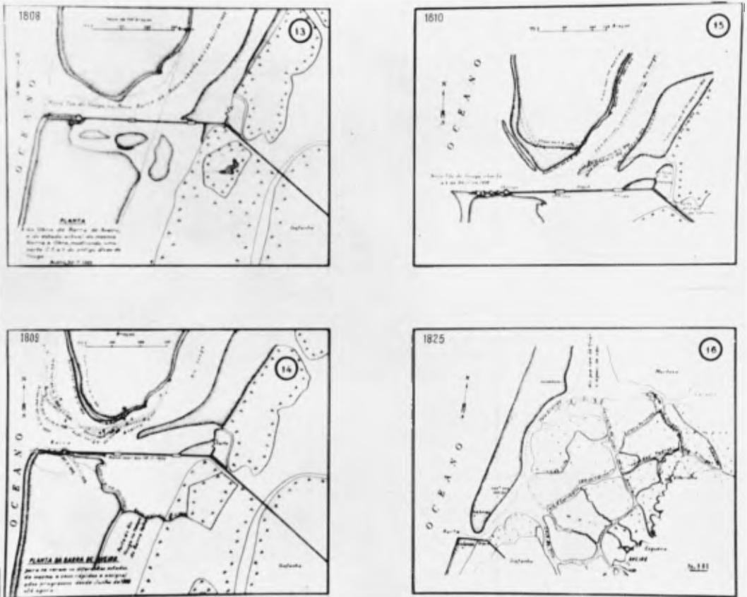
Fig. 5. Behavior of the artificial inlet up to 1825.
