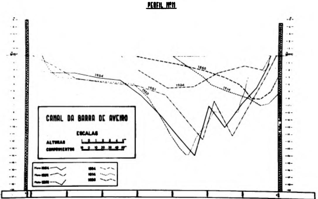
Fig. 29. Evolution of the inlet's channel cross-sections due to the works (range No. 11).
