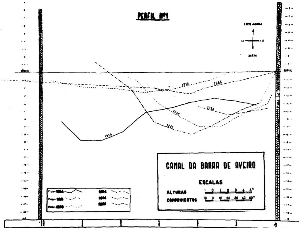
Fig. 27. Evolution of the inlet's channel cross-sections due to the works (range No. 1.).
