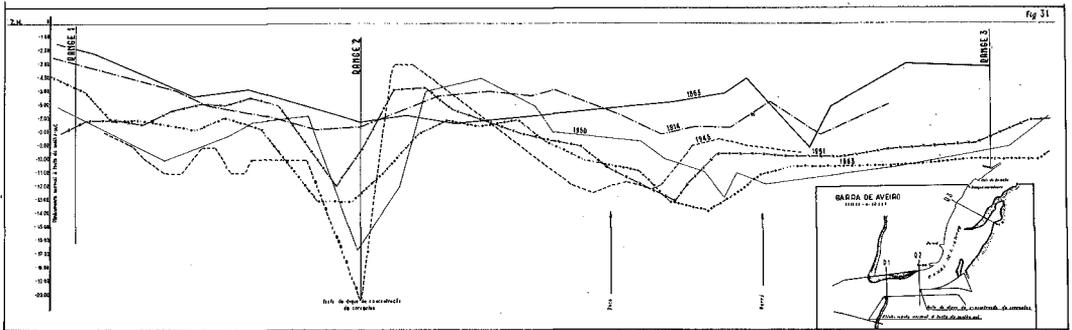
Fig. 31. Longitudinal profiles along the talweg between the inlet's mouth and S. Jacinto, from 1865 to 1953.
