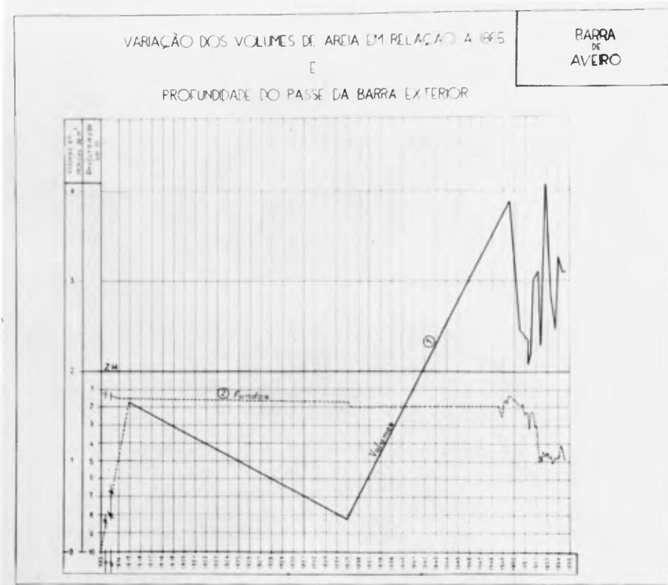
Fig. 22. Variation in the volume of the sand deposits over the outer bar (curve 1) and in the controlling depths over the same (curve 2), from 1865 to 1954.
