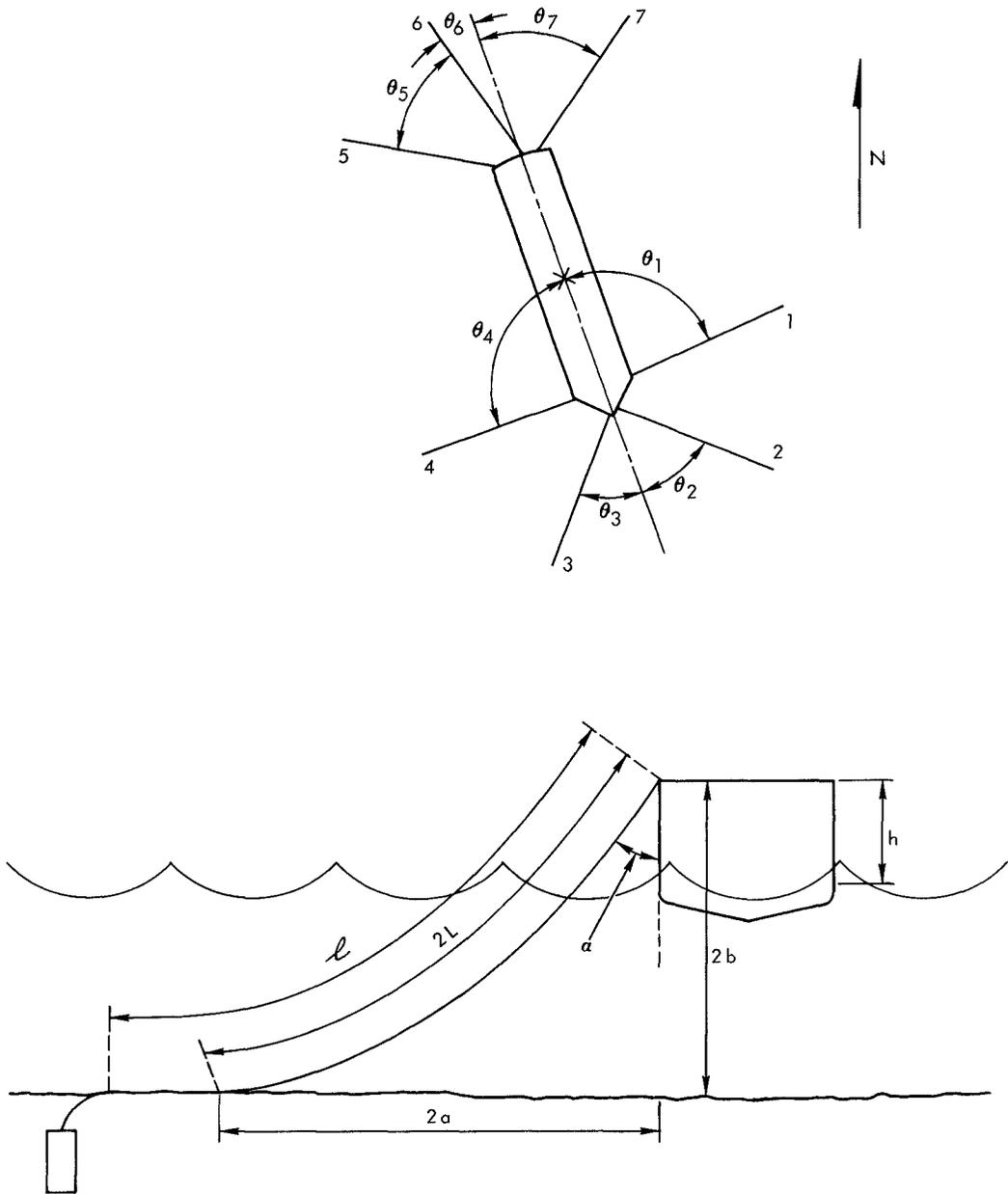
Figure 2 Convention used to describe mooring chain geometry.
