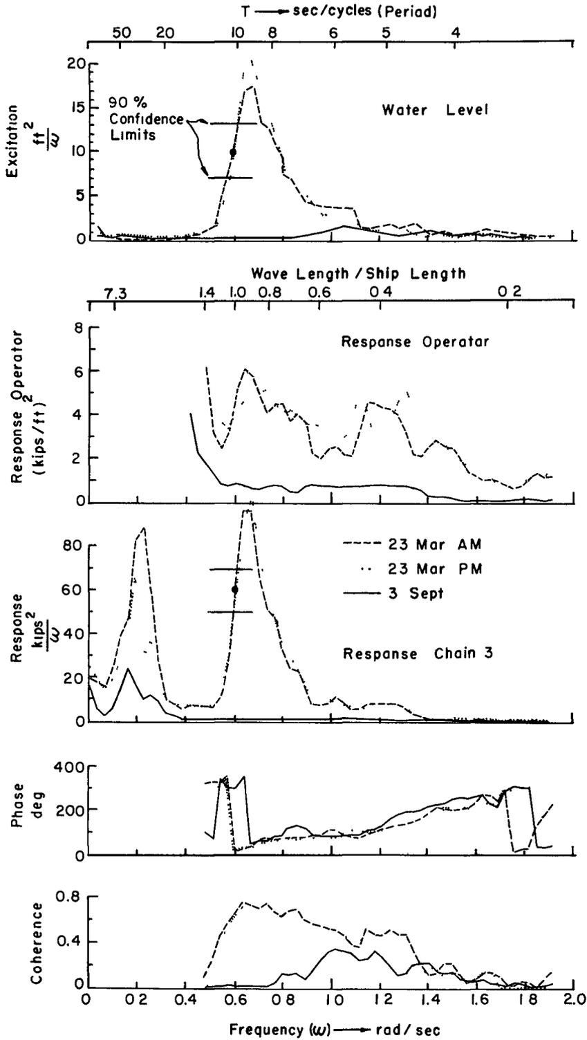
Figure 6 Water level versus tension in starboard bow-chain (No. 3). The phase convention is: Tension increase lags water level (wave) crest up.
