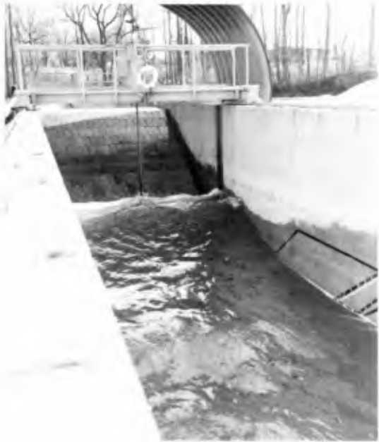
Fig. 7. Concrete block revetment in large wave tank.
