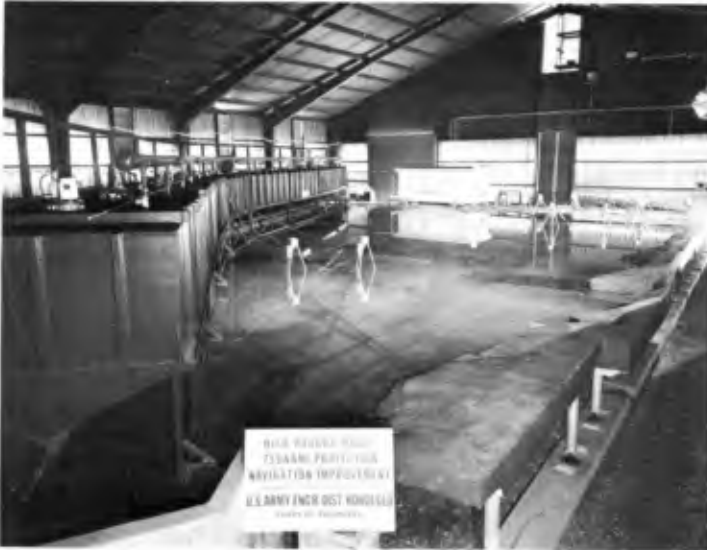
a. General view of Hilo Model looking south with wave generator at left, instrument room in center, and inner bay area on the far right.
