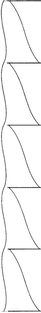
Fig 9 b DISTANCE BETWEEN GROYNES  $6L_g$  ,  $q_1 > q_2$
