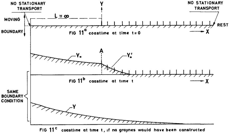
Assume, that by one or another external cause (for instance, a river or tidal canal, which embouches left of the left boundary, fig. 11) the coastline at time  $t$ , would have been according to fig. 11c, if no groynes would have been constructed.
