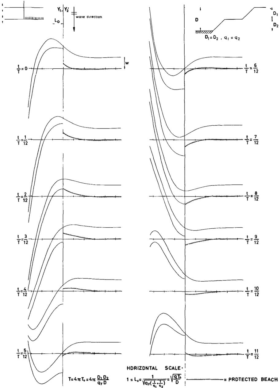
FIG 13 PROPAGATING SANDWAVE ACCORDING TO TWO-LINE SYSTEM
