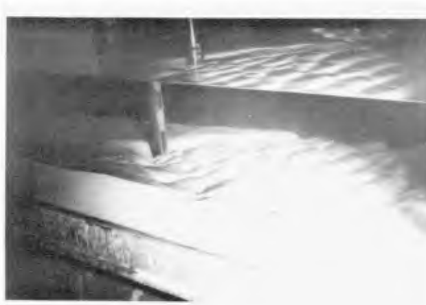
Fig. 10. SCOUR PATTERN WAVE NO. 1 - 8 inch depth, Sand No. 3
