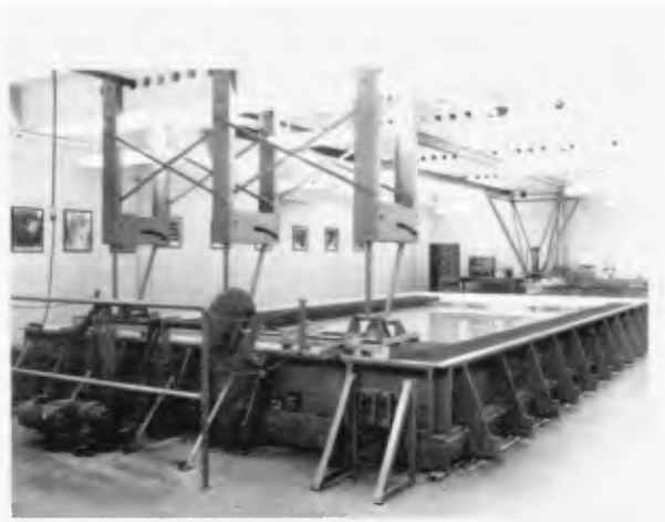
Fig. 3 Over-all view of the wave basin and wave generator with wave filter and absorbers in place
