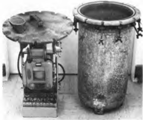
Fig. 11. INES wave recorder
