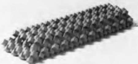
Pl. 1 The detached breakwaters on Ishizaki coast and the model of the hexa-leg-blocks
