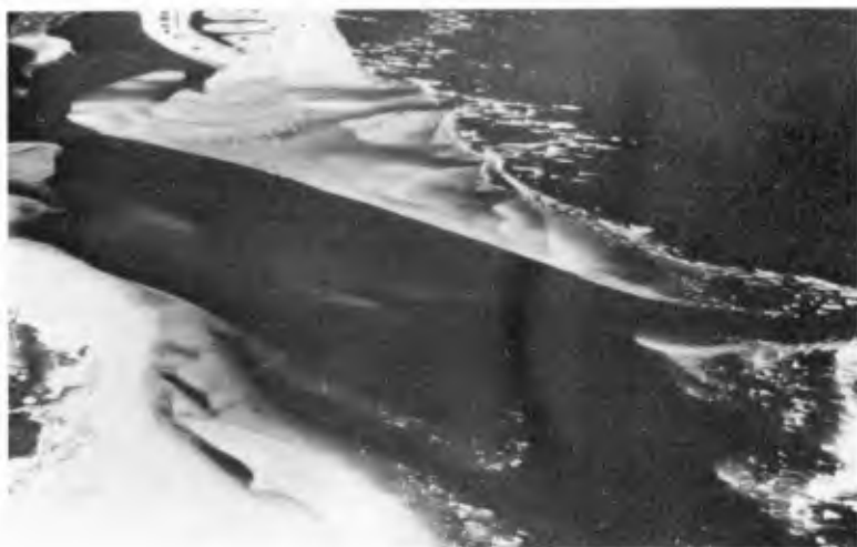
Figure 1. Low tide photograph of Murrells Inlet, S. C. Note the large shoal occupying the channel cross-section. This is a result of the near balance of sand moving in and out of the inlet.
