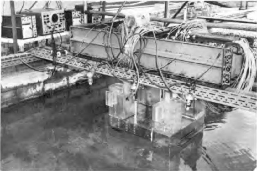
FIG. 7 Model Berth Caisson and instrumentation
