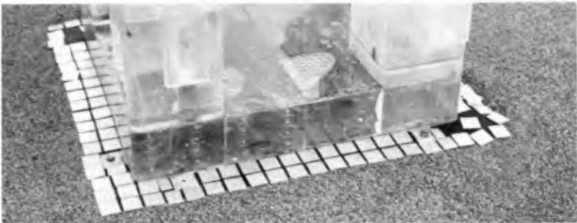
FIG. 12 Scour protection - 24 ft Waves from E.S.E. at L.W.
