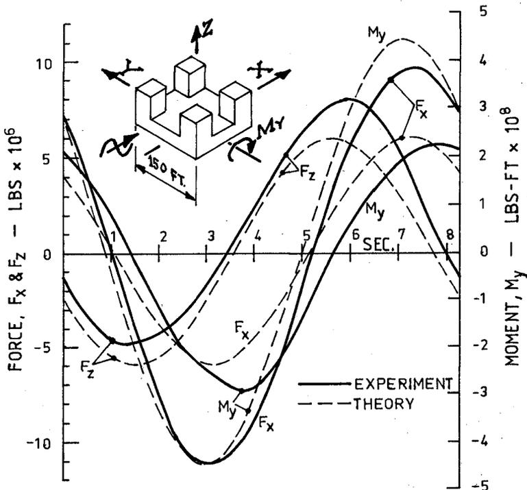
FIG. 6 WAVE FORCES FROM EXPERIMENT AND THEORY.
