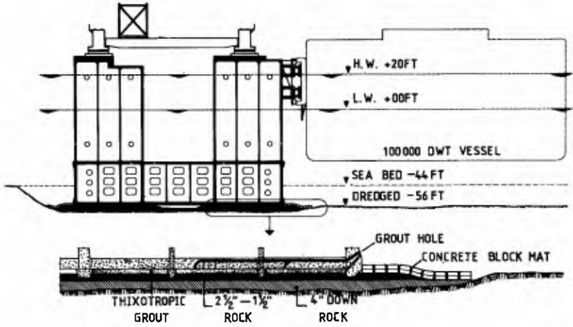
FIG. 3 Main Berth Caisson; structure and foundations
