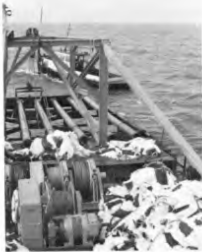
Fig. 7. Pontoon with the eight P.V.C. tubes in horizontal position.
