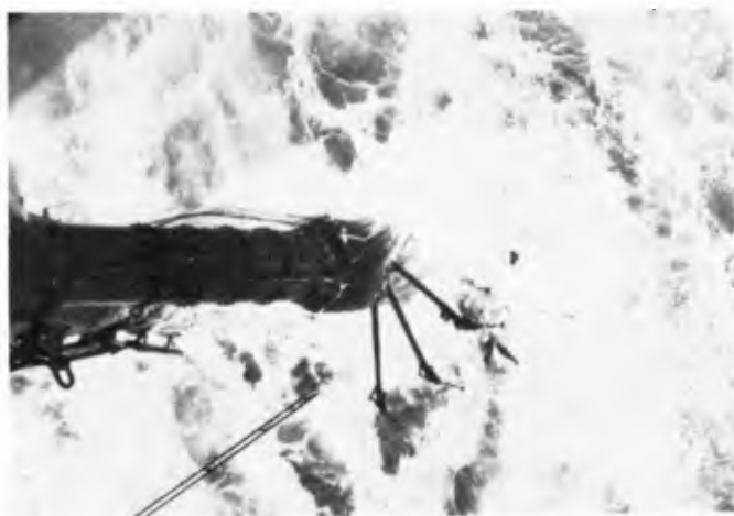
Fig. 2 : Test section clamped on on inclined member of the platform substructure to be seen on extremely low tide water level at storm conditions. Baylor wave staff on the left hand side.
