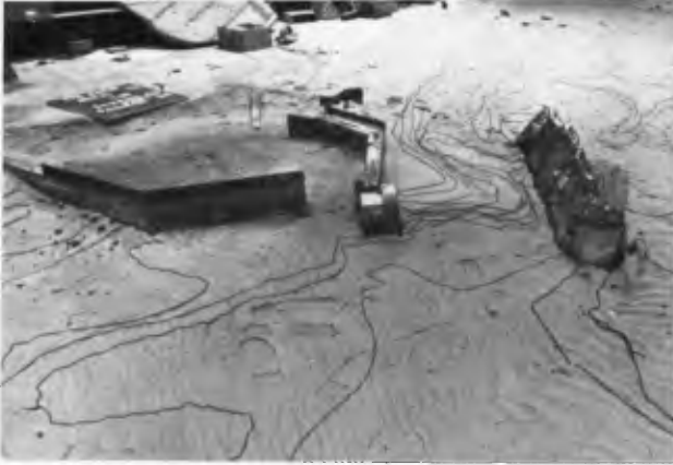
Fig. 6 Build-up in model sand trap
