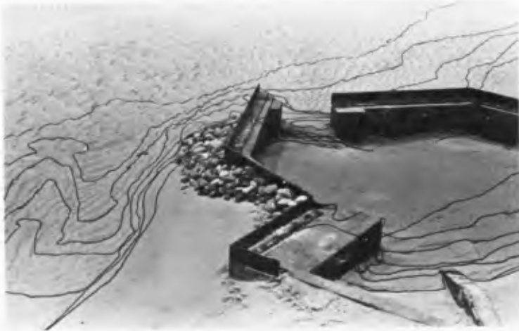
Fig. 4 Sand deposition in model harbour entrance
