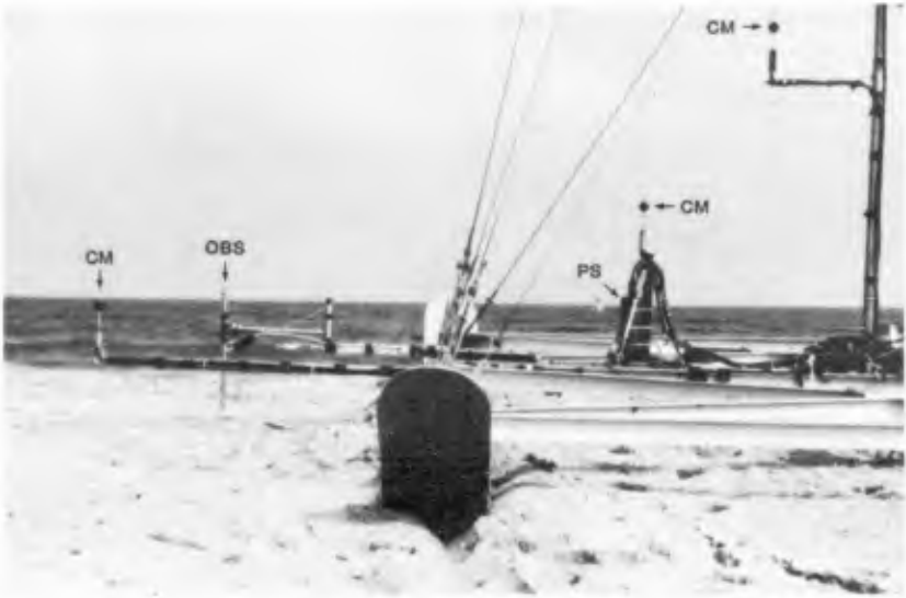
Fig. 3 Sled instrumentation. Shown are three current meters (CM), a pressure sensor (PS), and an array of optical backscatter (OBS) sensors (photo courtesy of Bruce Richmond).
