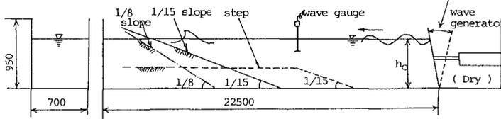
Fig.8 Schematic view of experimental set-up
