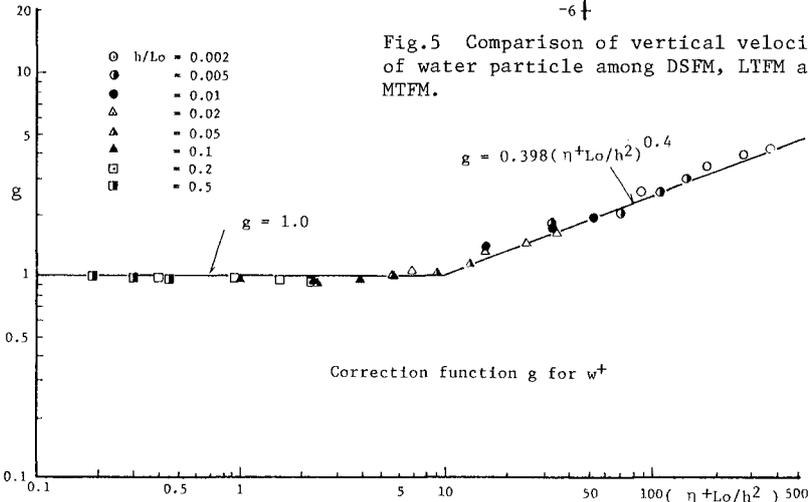
Fig. 6 Value of correction function  $g$  for  $w^+$ .
