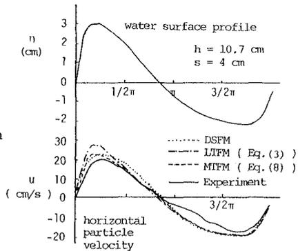
Fig.1 Comparison between measurement and calculations (Regular wave; experimental and DSFM's values are from Nadaoka et al.<sup>4</sup>).
