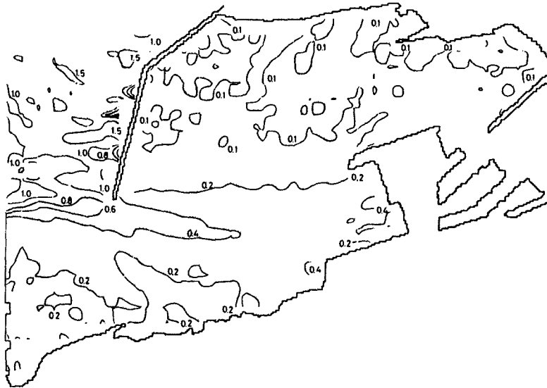
Fig.9: Isolines of variance for the wave propagation problem in the new Bilbo Harbour (Superport).
