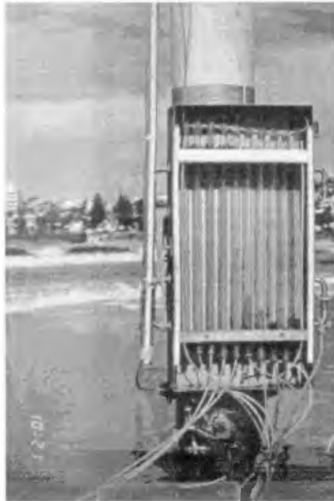
Figure 4: The "barometer" mounted on the stilling well which served as a bench mark for the surveys for reference it can be compared with the schematic representation in Figure 5.
