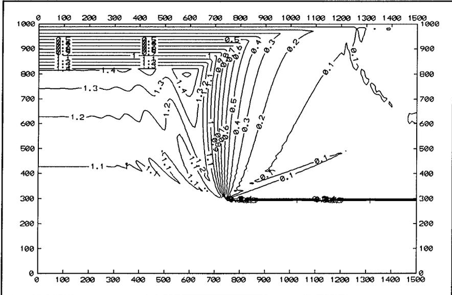
Figure 7.- Wave height field for monochromatic test
