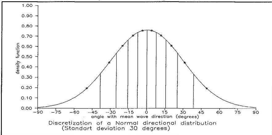
**Figure 1.- Equalized discretization for a directional shape.**
