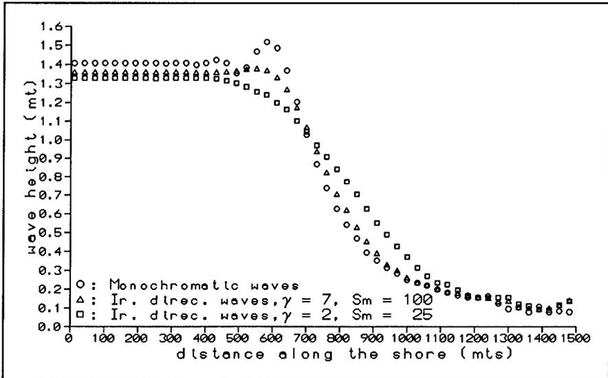
Figure 10.- Breaking wave height along the shore
