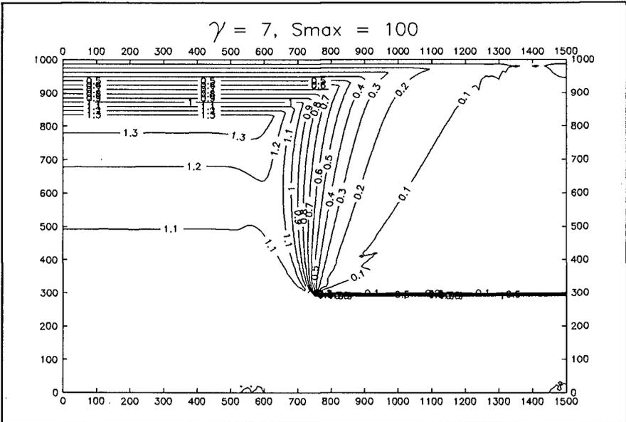
Figure 8.- Wave height field for swell conditions test
