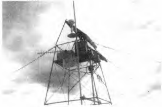
Figure 2 Details of the tower. From left to right; the aerial to send back the data by telemetry. The box with batteries the radio and the electronics box for the ZWARTS pole, just in front the anemometer mast and the hydrometer, on top the solar cell, and on the back side the ZWARTS pole.
