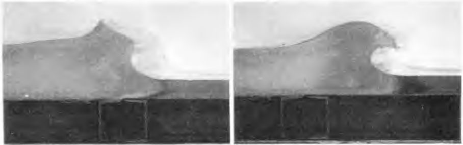
Photo 1 : Snapshots of the composite breaker from the generation of the 2nd crest to the jet-fall initiation
