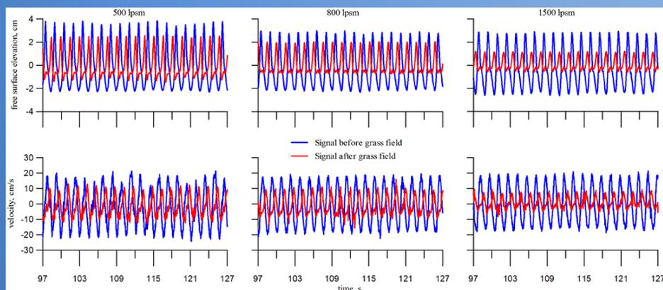
Figure 1 Comparison between transmitted and incident free surface signals (top) and velocities measured before and after the seagrass model (bottom).
