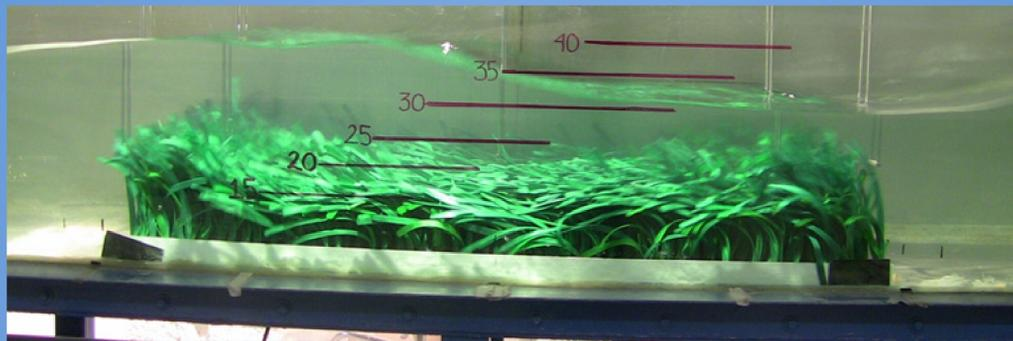
The wave conditions inside the flume were measured by 9 wave gauges. Incident, reflected and transmitted waves were the main values of interest. In addition, two Vectrinos were settled to get a view of the velocities prior to and after the seagrass.
