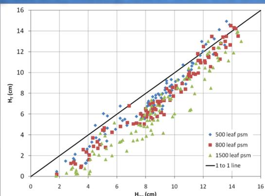
Figure 2 Comparison of incident and transmitted waves
