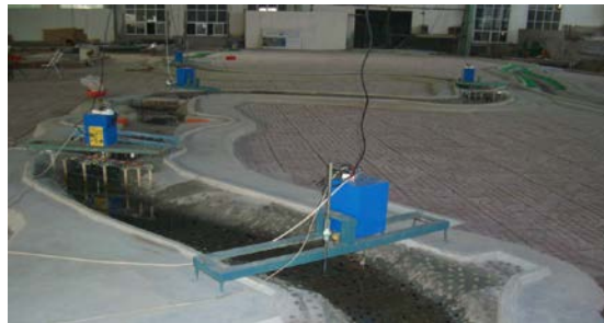
Figure 3. Photo of physical model of Mulanxi River.
