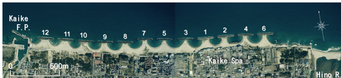
Figure 2. Aerial photograph of beaches around twelve detached breakwaters of Kaike coast taken in 2003.
