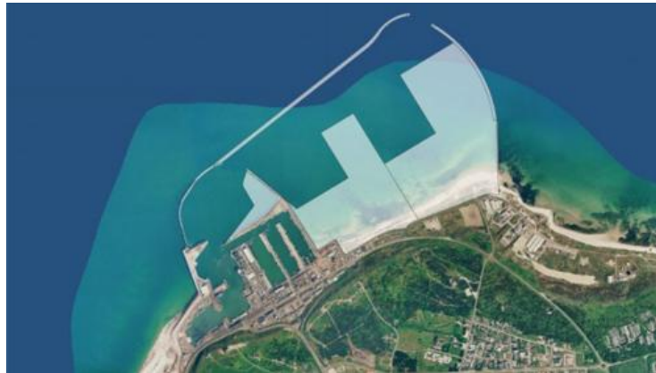
Figure 2. Planned extension of the Port of Hanstholm. The existing harbour forms the east part of the future harbour.
