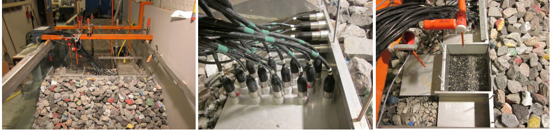
Figure 6. (left) Front view of breakwater, (middle) Pressure transducers in static part of crown-wall, (right) Moveable part of crown-wall.
