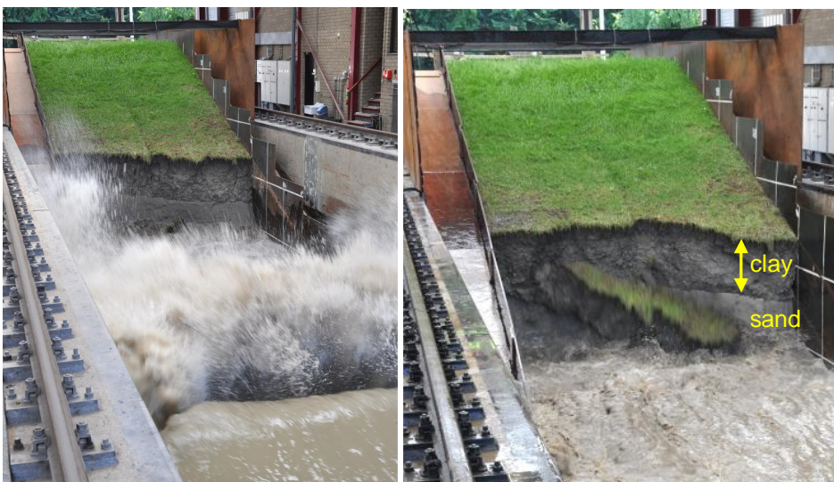
Figure 11, Erosion process: undermining of the clay layer
