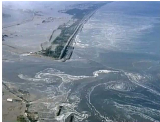
Photo 15. Return flow in the sea issued from the breach point, the right bank of the Abukuma River mouth, at 16:33 JST, captured from "Michinokugo" video.
