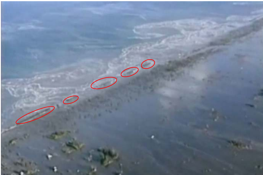
Photo 23. Return flows from the break points on southern Yamamoto Coast, at 16:39 JST, March 11, shot from "Michinokugo". Upper left of the photo is the sea. Encircled objects are levees above the sea surface.
