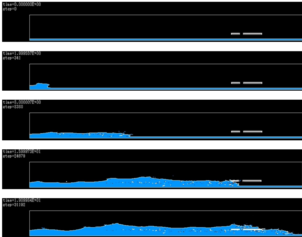
Figure 5. Snapshots of tsunami propagation in numerical wave tank.
