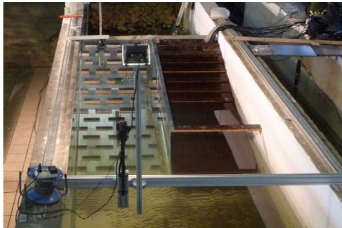
Figure 11. Model set-up (here: configuration p0r2) in the 2m-wave flume of Leichtweiss-Institute
