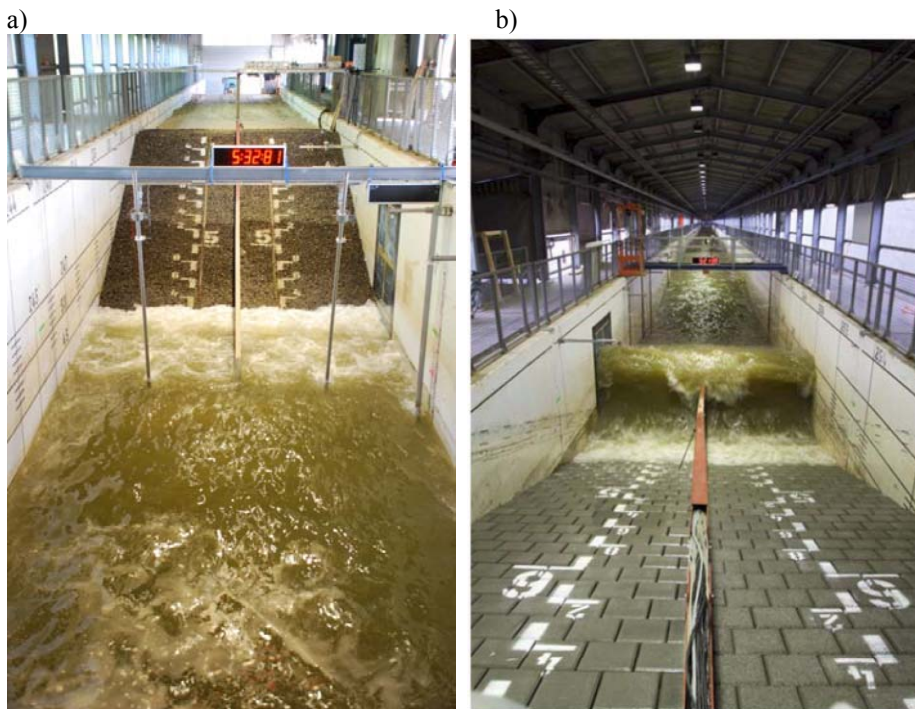
Figure 4. Photos of the different revetments under wave attack in GWK: a) PBA revetment (Oumeraci et al. 2010), b) IPPB revetment (Gier et al. 2011)
