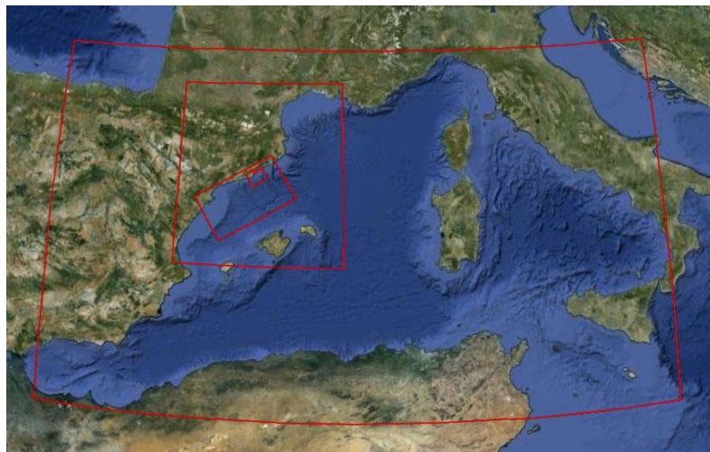
Figure 2. Distribution of numerical modelling domains, covering the full western Mediterranean (to generate realistic offshore boundary conditions) and nested till reaching the topographic and bathymetric “details” along the Catalan coast.
