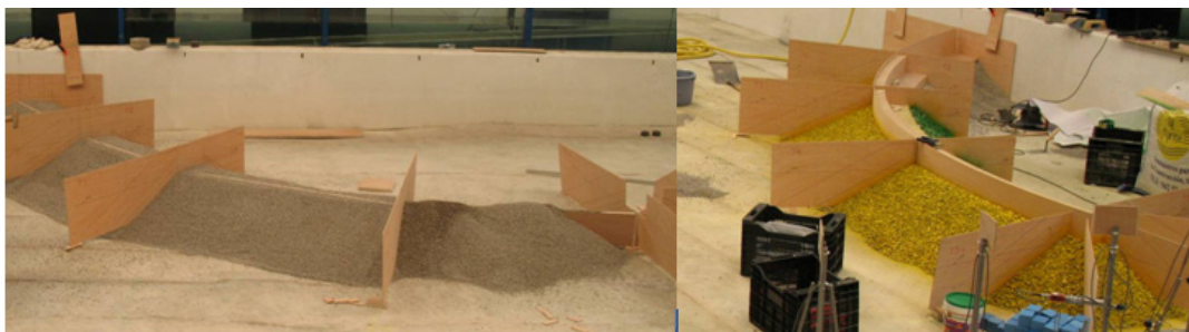
Figure 5. Transversal sections of the scaled structure for the stability test in laboratory.
