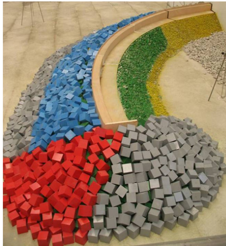
Figure 6. Final layout of the rubble-mound breakwater constructed. 60 Ton cubes (grey and blue) y 70 Ton cubes (red).
