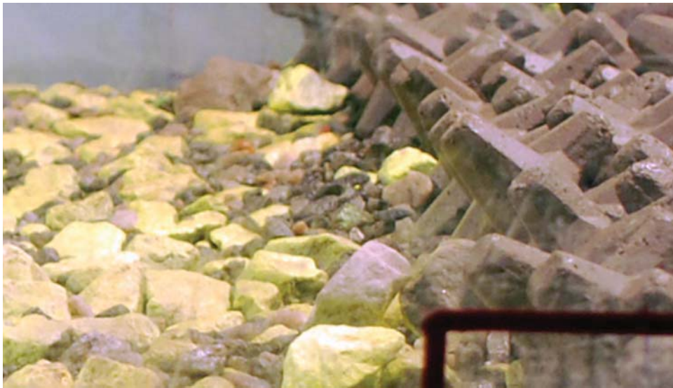
Figure 13: Outermost row of toe reinforcement – showing accumulation of smaller quarry run rock after test
