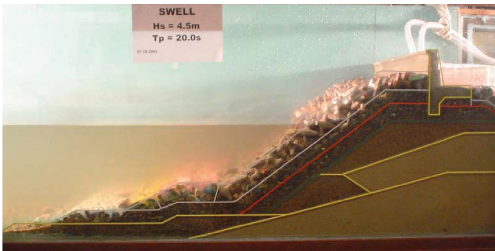
Figure 4: Toe Berm at -8.3m LWOST, Revetment slope 4:3, Toe Apron thickened for geotechnical stability
