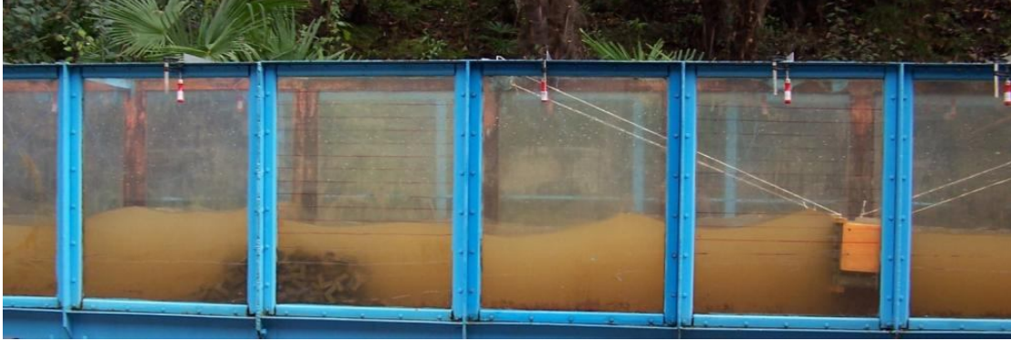
Figure 16. Decomposition of initial waves after second bar and its absorbing by floating breakwater.
