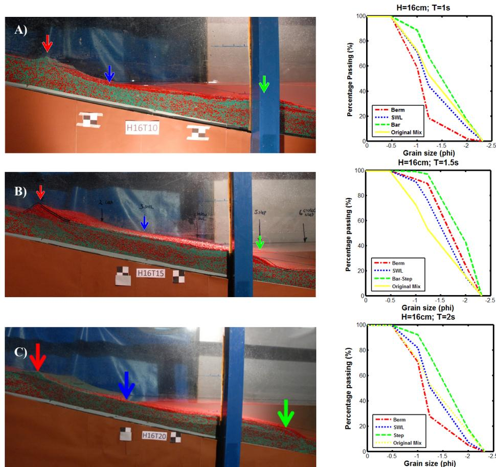
Figure 6. Left panels show a beach profile pictures and right panels the sediment distribution curve for the position of the berm, shoreface and bar/bar-step. A) Test H16T10, B) Test H16T15, C) H16T20.
