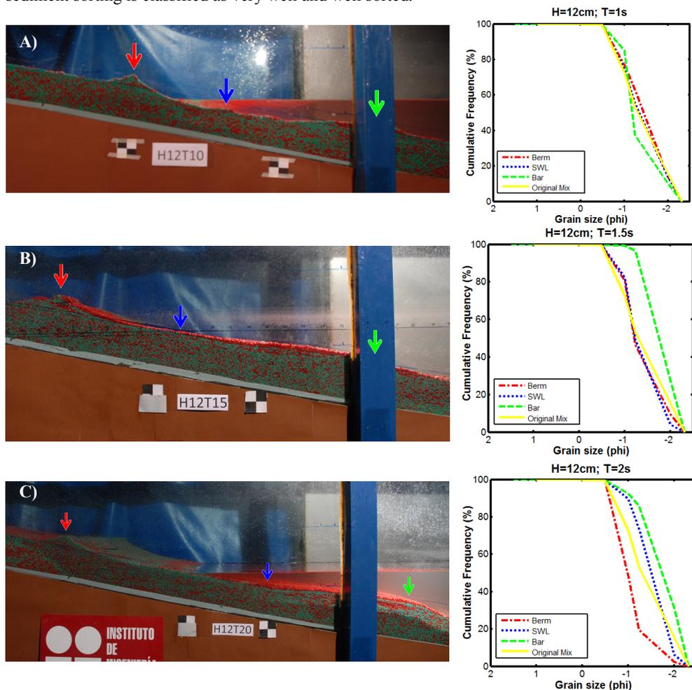
Figure 5. Left panels show a beach profile photography and right panels the sediment distribution curve for the position of the berm, shoreface and bar/bar-step. A) Test H12T10, B) Test H12T15, C) H12T20.
