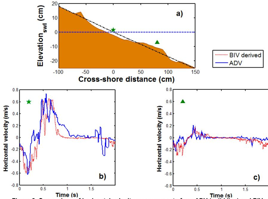
Figure 8. Comparison of horizontal velocity measurements from ADV (solid line) and BIV (dots). Panel a: illustrate the position of the point of analysis; Panel b: illustrate a point of analysis near swl; Panel c: illustrate point of analysis over the bar.
