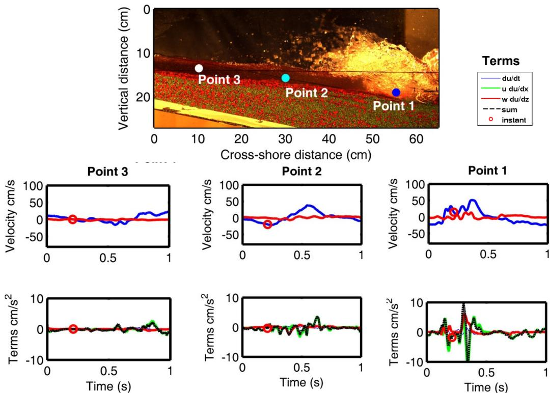
**Figure 9.** Test  $H=0.16\text{ m}$ ,  $T=1\text{ s}$ . Top panels illustrate the points of evaluation. Middle panels show velocities vertical (blue) and horizontal (red); Bottom panels show advective terms (horizontal in green, vertical in red), local terms (blue) and the sum (gray).
