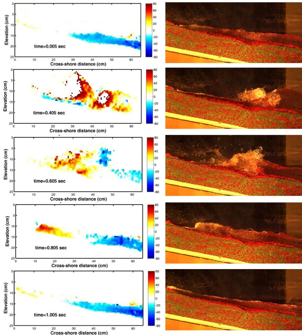
Figure 7. Snapshots of a plunging wave ( $H=0.12$  m;  $T=1.0$  s) travelling on the permeable slope (right panels) and BIV derived horizontal velocity fields in cm/s (left panels).
