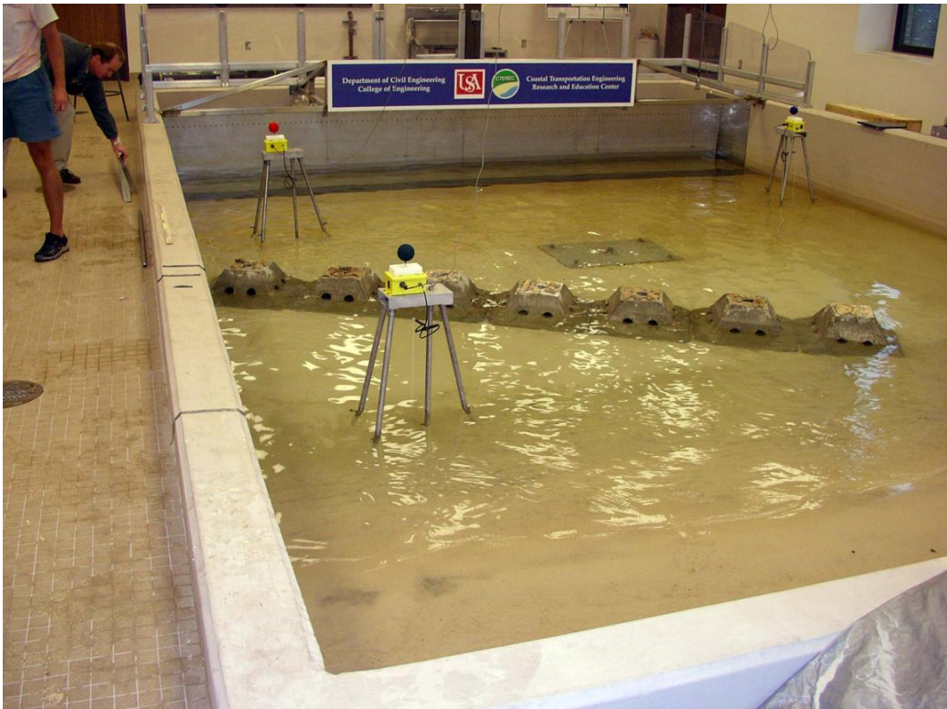
Figure 12. The University of South Alabama wave basin during 1:5 scale model wave transmission tests of the so-called “Wave Attenuation Devices” or WADs eventually used in the Little Bay project breakwater. The test configuration shown is a single row of concrete units aligned obliquely to the incident waves.
