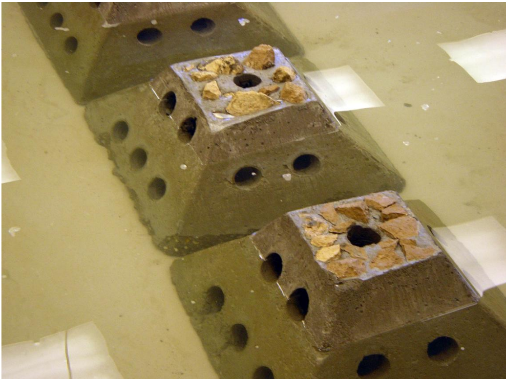
Figure 13. A close-up photograph of the scale model concrete units called “Wave Attenuation Devices, or WADs,” in the laboratory basin.
