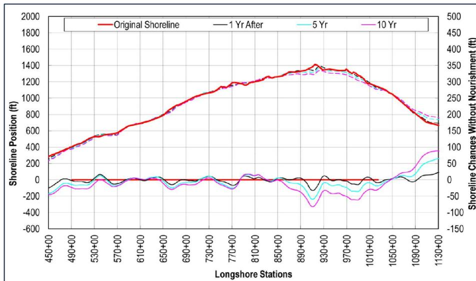
Figure 8. Predicted shoreline positions and changes in 1 year, 5 years, and 10 years without nourishment. [Note: The upper group of lines represent shoreline positions at various run times, and the lower group of lines represent corresponding shoreline changes relative to the original shoreline position (ie — 2009 shoreline).]
