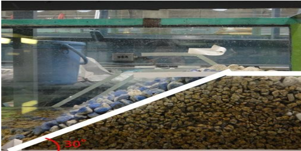
Figure 4. Experimental layout of the breakwater
