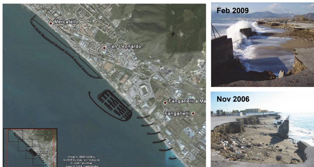
Figure 3. Gulf of Salerno coastal protection scheme and example of coastal erosion
